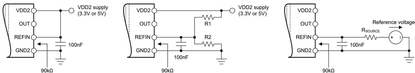
Figure 8-3. Connecting the REFIN Pin
