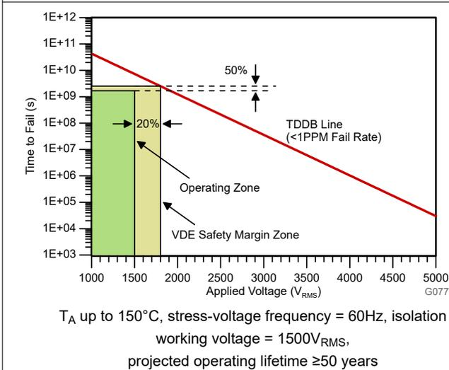
Figure 6-4. Isolation Capacitor Lifetime Projection (Reinforced Isolation)
