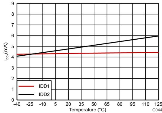
Figure 6-14. Supply Current vs Temperature
