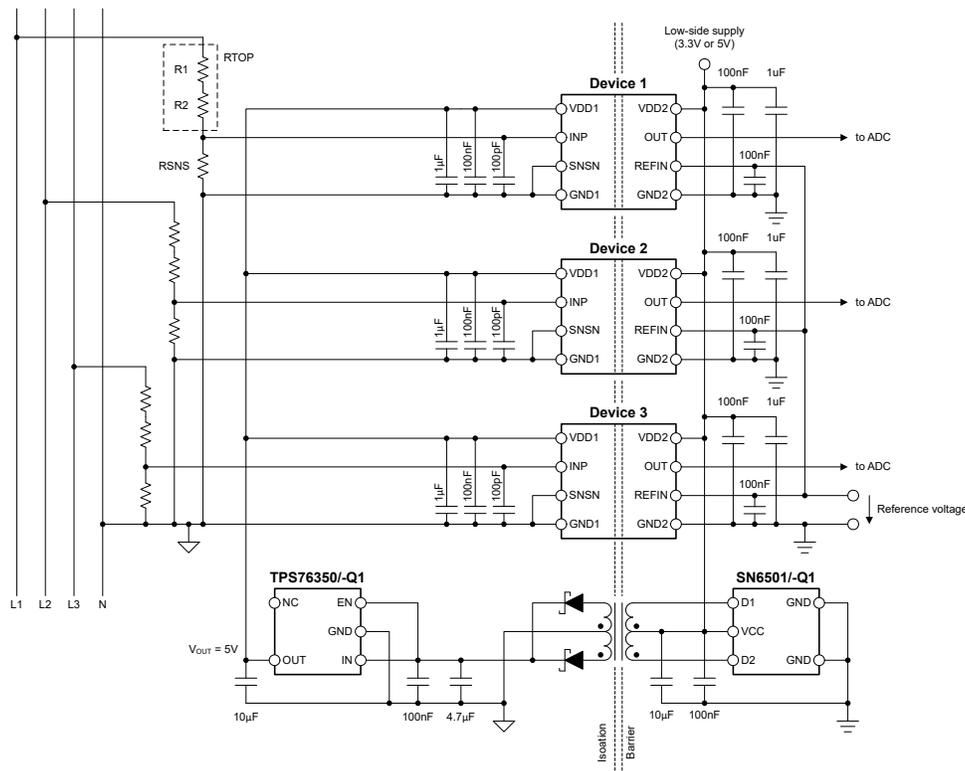
Figure 8-1. Using the AMC0x30R-Q1 in a Typical Application
