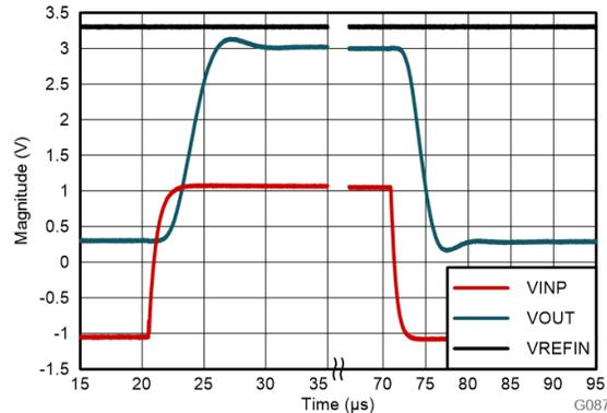
**Figure 8-4. Step Response of the AMC0x30R-Q1**
