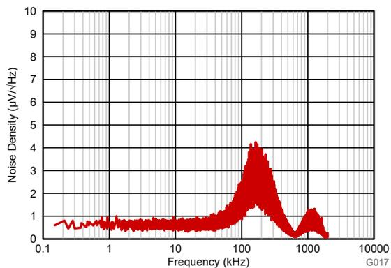
**Figure 6-10. Input-Referred Noise Density vs Frequency**
