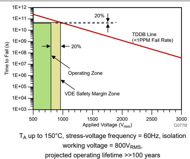
Figure 6-5. Isolation Capacitor Lifetime Projection (Basic Isolation)
