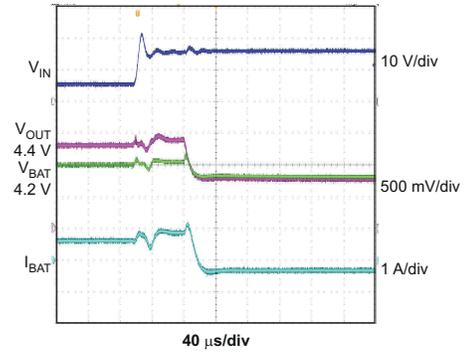
$V_{IN} = 6\text{ V to }15\text{ V}$        $R_{LOAD} = 10\ \Omega$
