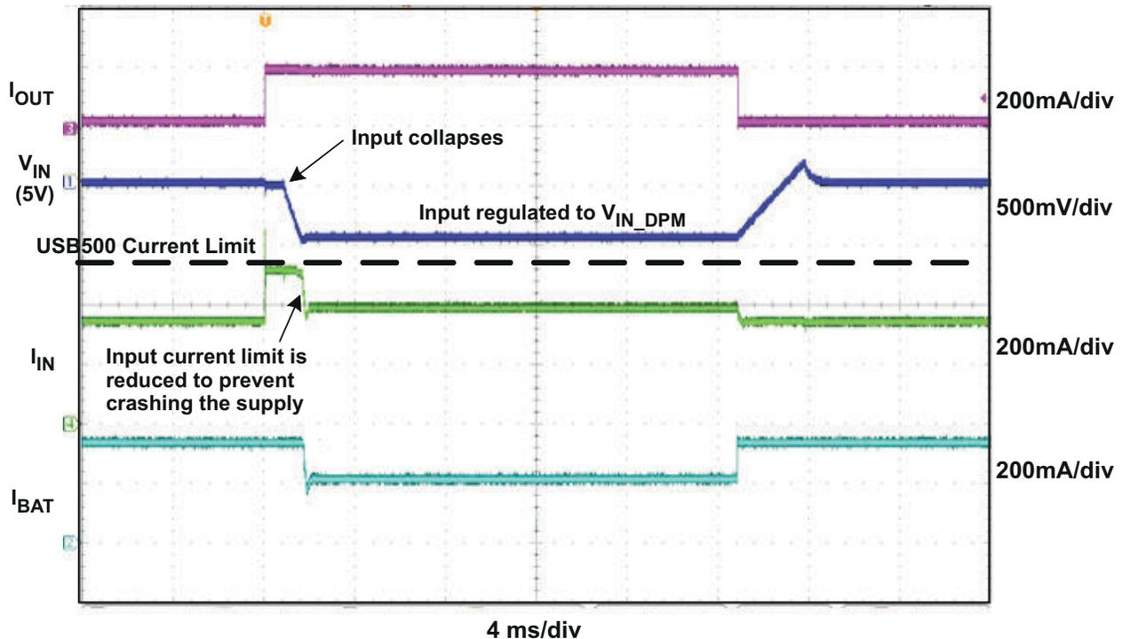
Figure 9-3.  $V_{IN-DPM}$  Waveform
