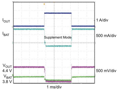
$R_{LOAD} = 25 \Omega$  to  $4.5 \Omega$
