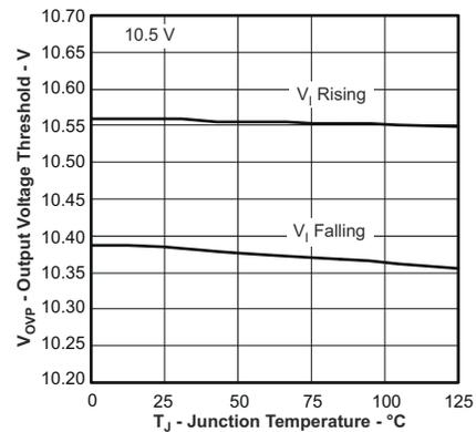
Figure 8-10. BQ24074 Overvoltage Protection Threshold vs Temperature
