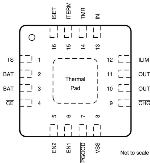
**Figure 7-2. BQ24074 RGT0016B Package 16 Pins Top View**
