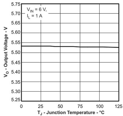
Figure 8-7. BQ24075, BQ24079 Output Regulation Voltage vs Temperature
