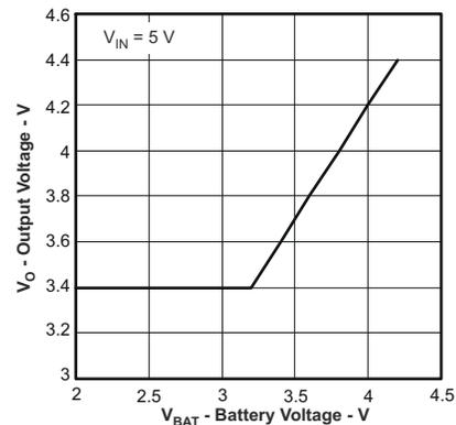
Figure 8-4. BQ24072 Output Regulation Voltage vs Battery Voltage
