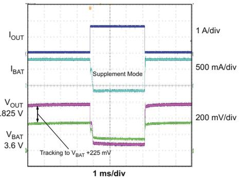
$R_{LOAD} = 20 \Omega$  to  $4.5 \Omega$
