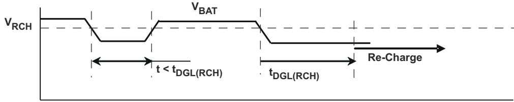
Figure 9-12. Recharge –  $t_{DGL(RCH)}$
