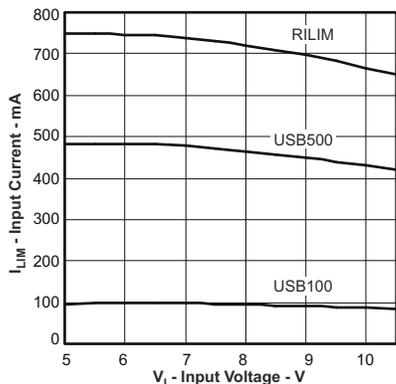
Figure 8-11. BQ24074 Input Current Limit vs Input Voltage
