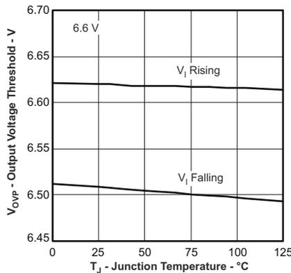
Figure 8-9. BQ24072/ 73/ 75/ 79 Overvoltage Protection Threshold vs Temperature
