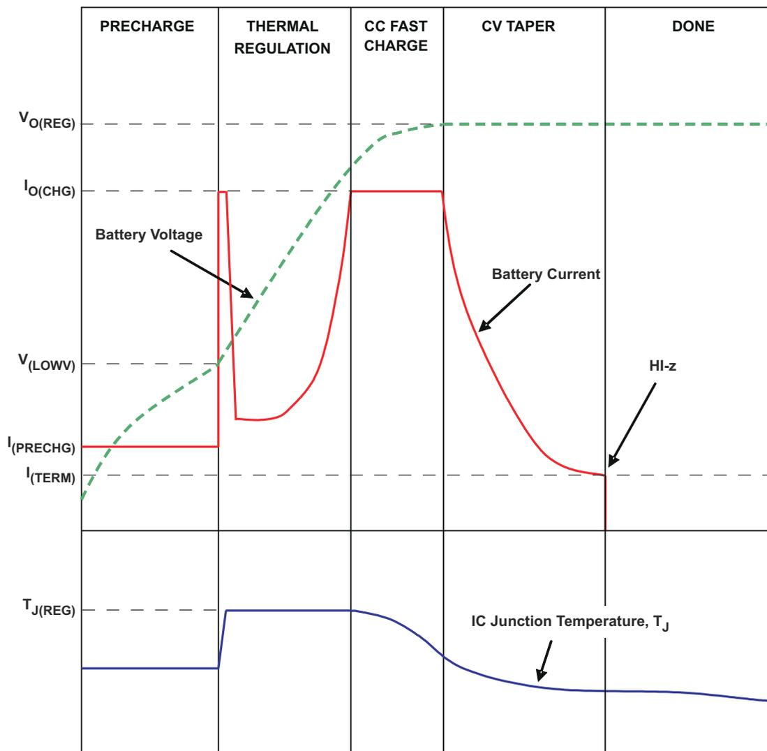
**Figure 9-8. Charge Cycle Modified by Thermal Loop**
