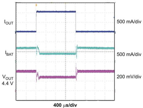
$R_{LOAD} = 20 \Omega$  to  $9 \Omega$
