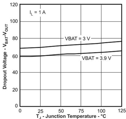
Figure 8-3. Dropout Voltage vs Temperature No Input Supply
