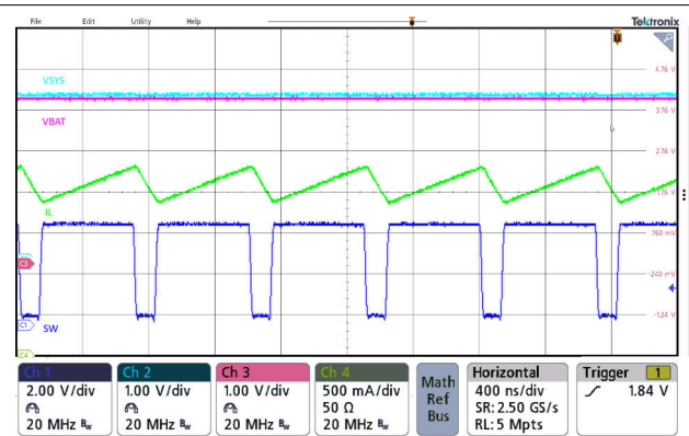
Figure 9-7. Charge Disable via \overline{CE} Pin
