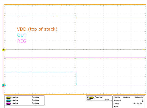
Figure 8-5. Overvoltage Protection Recovery
