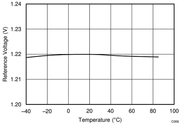
**Figure 7-4. Reference Voltage vs. Temperature**
