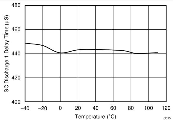
Threshold setting is 465 µs (including internal delay).
