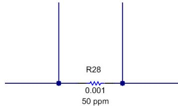
**Figure 9-5. Sense Resistor**
