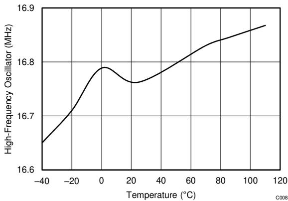
**Figure 7-6. High-Frequency Oscillator vs. Temperature**
