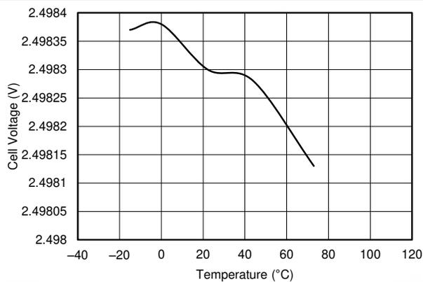
**Figure 7-14.  $V_{CELL}$  Measurement at 2.5-V vs. Temperature**
