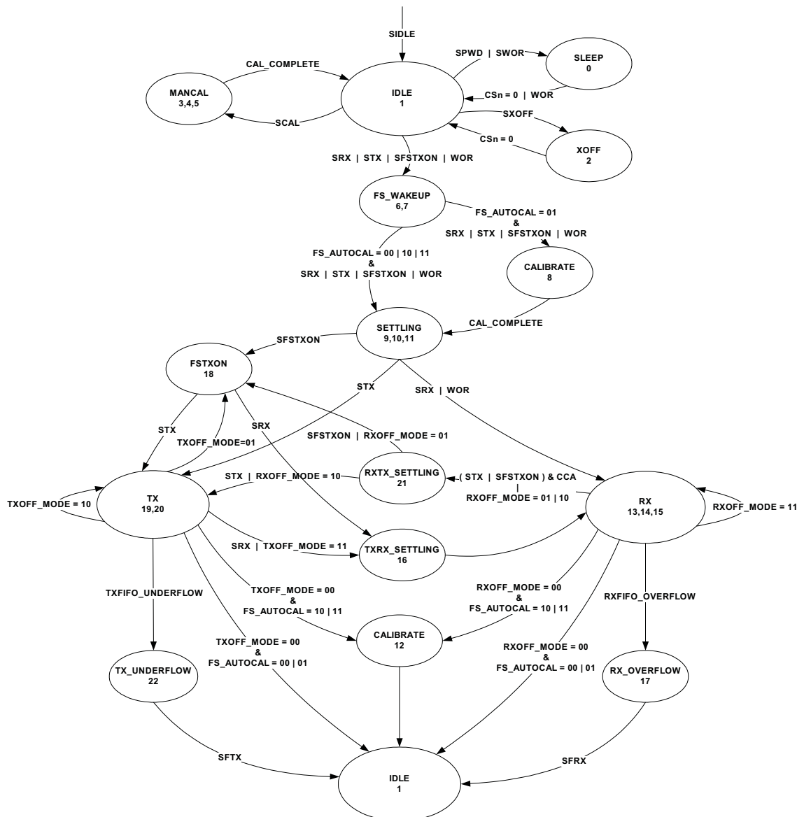
Figure 3-15. Complete Radio-Control State Diagram
