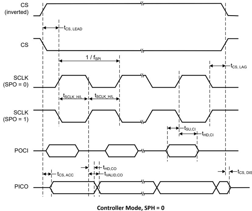
Figure 7-1. SPI Timing Diagram—Controller Mode, SPH = 0
