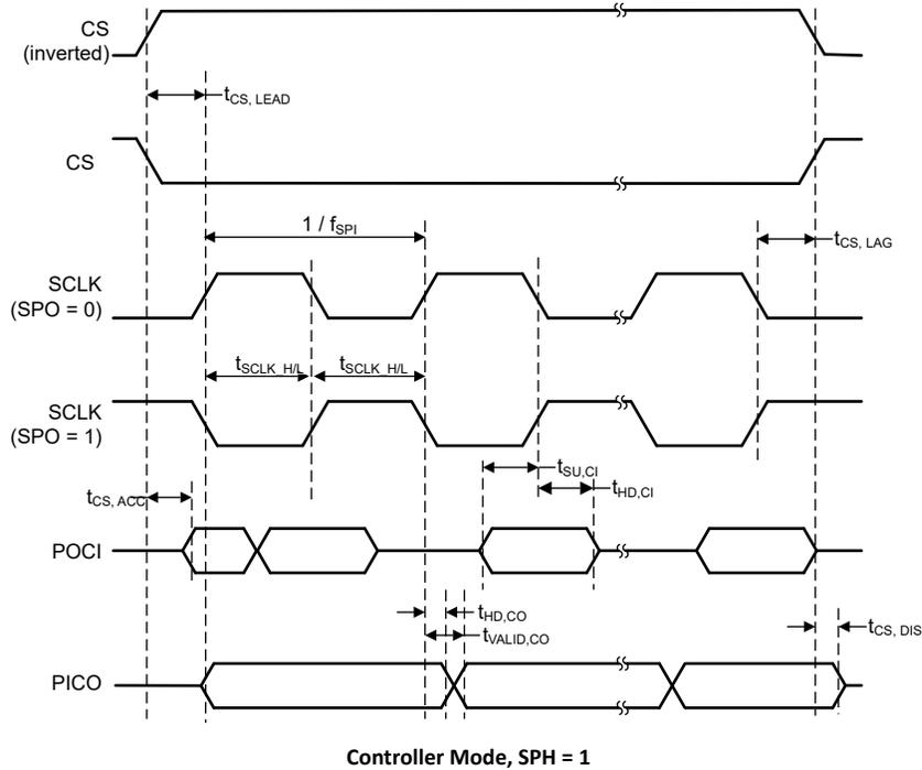
Figure 7-2. SPI Timing Diagram—Controller Mode, SPH = 1
