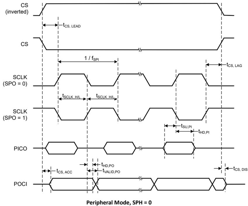
Figure 7-3. SPI Timing Diagram—Peripheral Mode, SPH = 0
