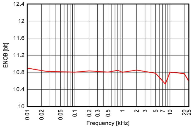
**Figure 7-27. ENOB vs. Input Frequency (Internal Reference)**
