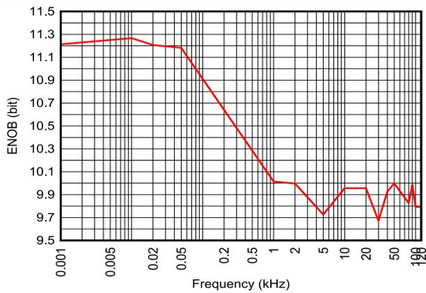
**Figure 7-29. ENOB vs. Input Frequency (External Reference = 3.0V)**
