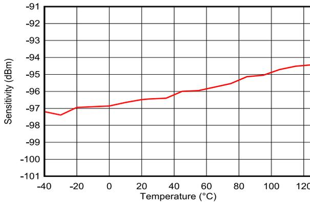
**Figure 7-16. Sensitivity vs. Temperature (Bluetooth LE 1Mbps, 2.44GHz)**
