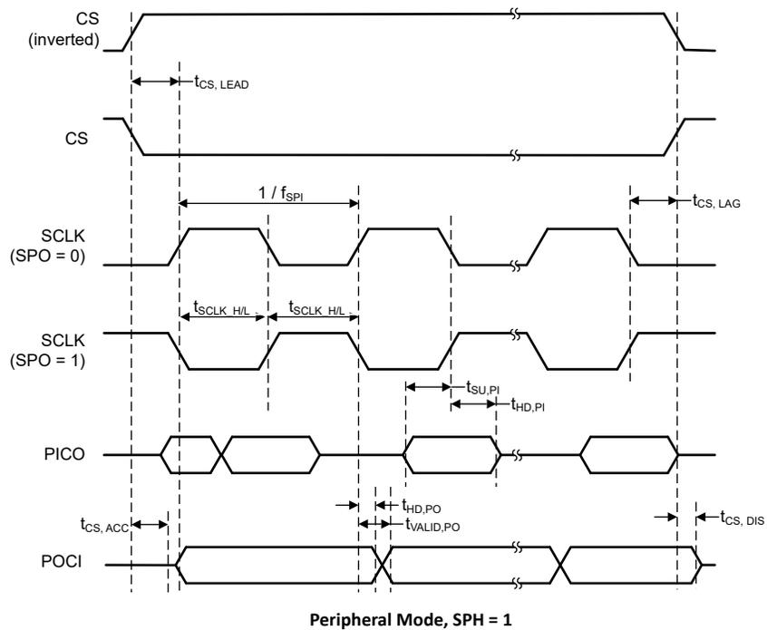
Figure 7-4. SPI Timing Diagram—Peripheral Mode, SPH = 1
