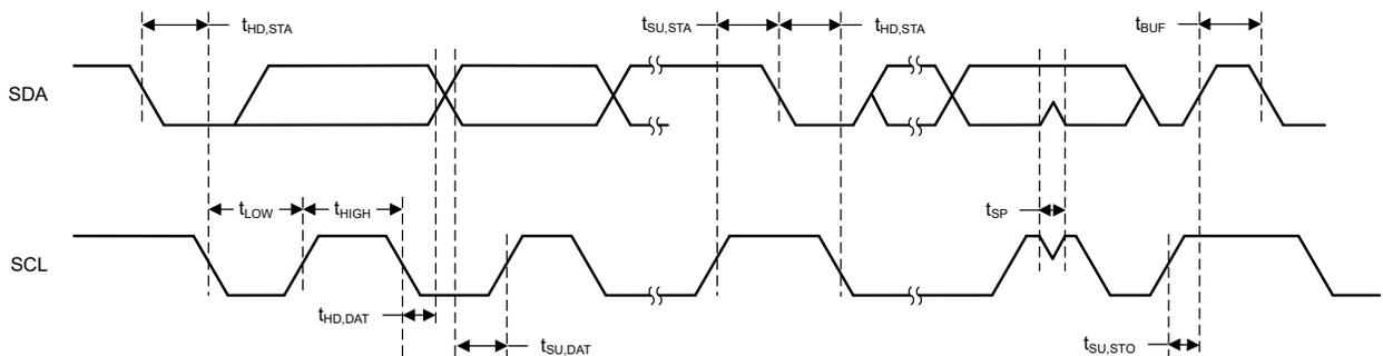
Figure 7-5. I<sup>2</sup>C Timing Diagram
