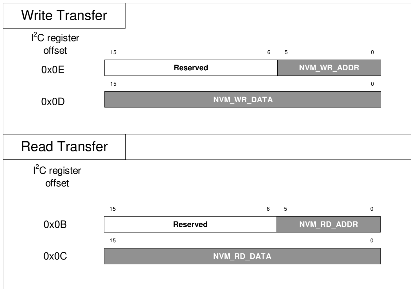
Figure 7-12. EEPROM Direct Access Using I 2 C
