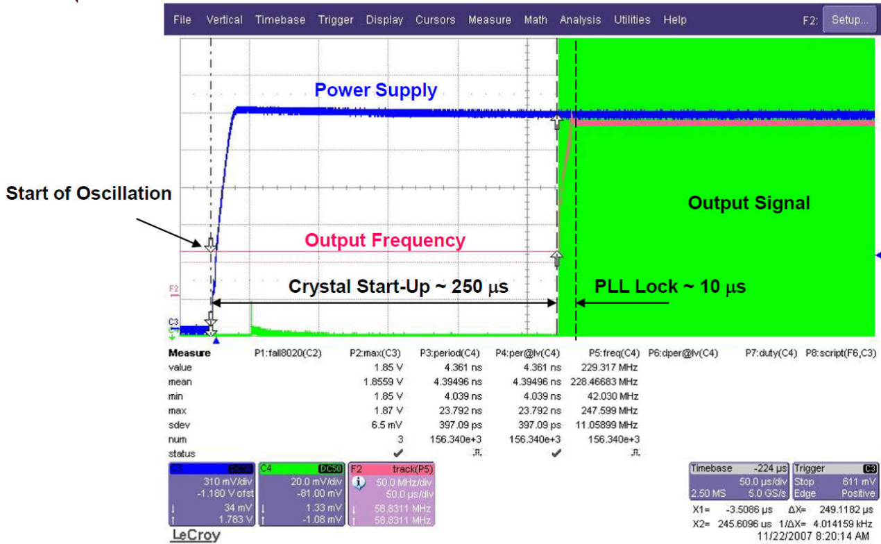
Figure 8-5. Crystal Oscillator Start-Up vs PLL Lock Time
