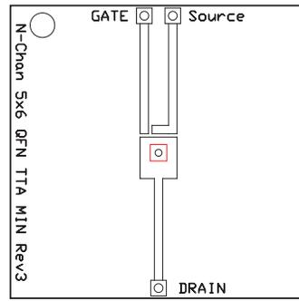
Max  $R_{\theta JA} = 120^{\circ}\text{C/W}$
