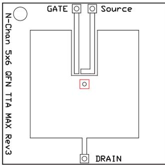
Max  $R_{\theta JA} = 50^{\circ}\text{C/W}$
