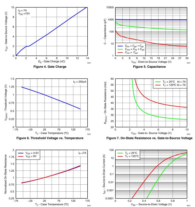
Figure 8. Normalized On-State Resistance vs. Temperature
