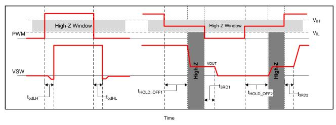
Figure 13. PWM Tri-State Timing Diagram
