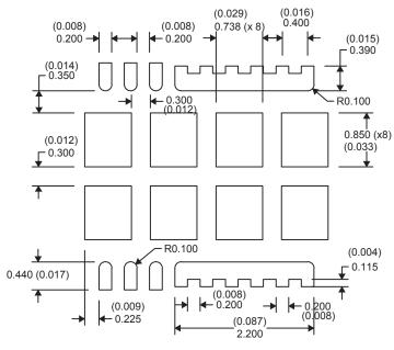
NOTE: Dimensions are in mm (inches). Stencil is 100µm thick
