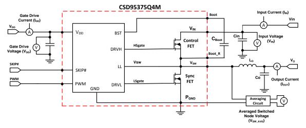
Figure 14. Power Loss Test Circuit
