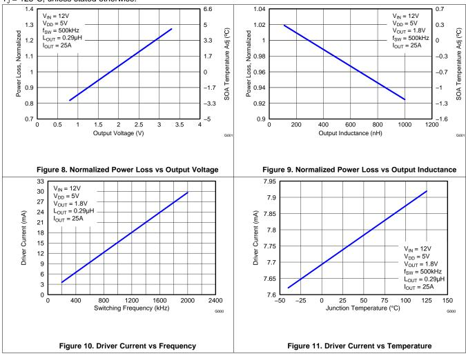
The Typical CSD95375Q4M System Characteristic curves are based on measurements made on a PCB design with dimensions of 4"
