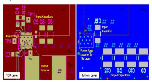
Figure 16. Recommended PCB Layout (Top Down View)
