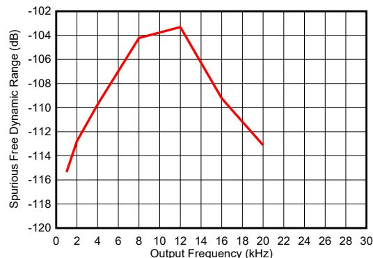
Figure 6-46. Spurious Free Dynamic Range vs Output Frequency, f_{DAC} = 768\text{ kHz}
