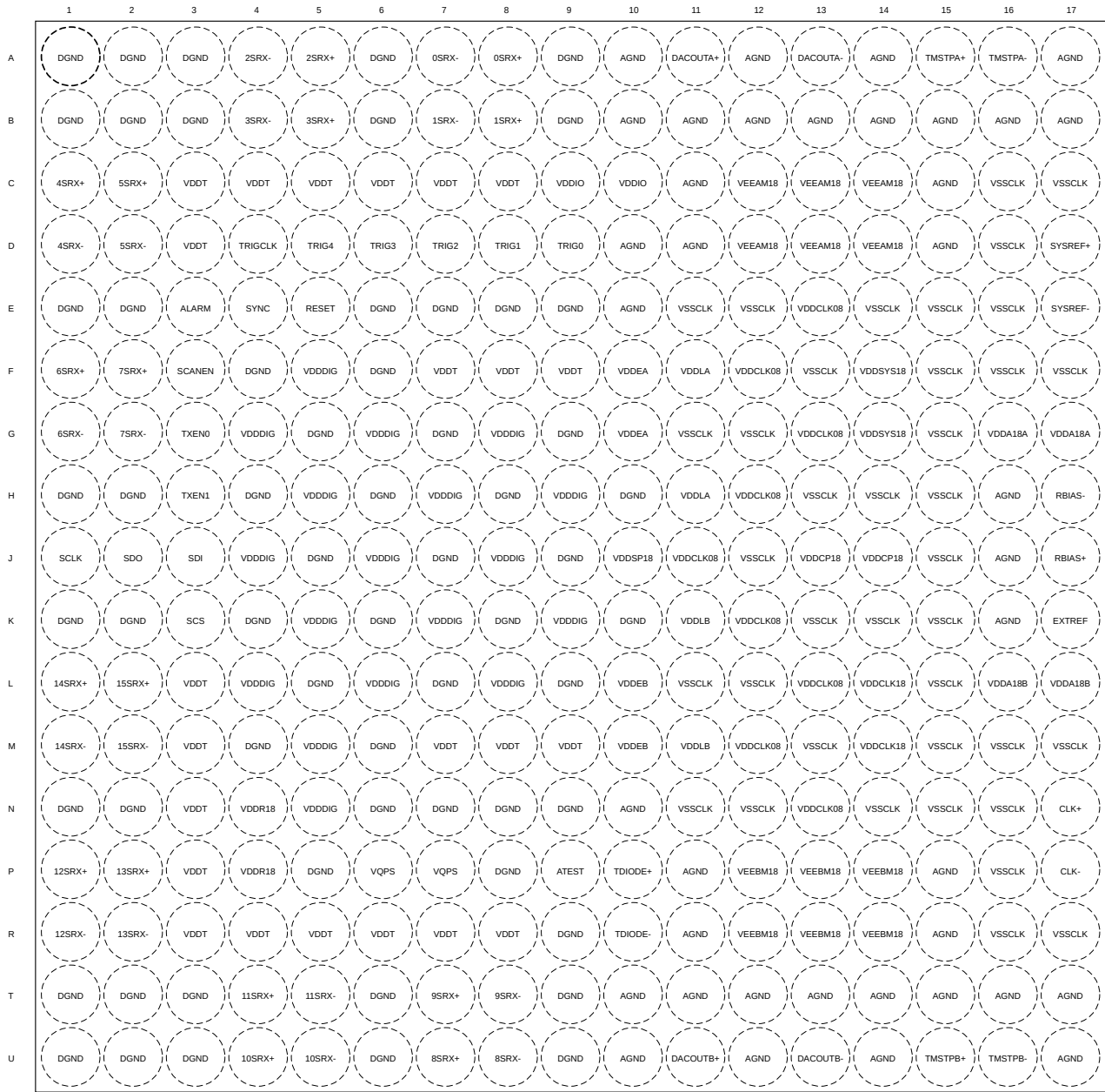
Figure 5-1. ANH0289A Package, 289-Ball Flip Chip CSP with 0.8mm pitch (Top View)
