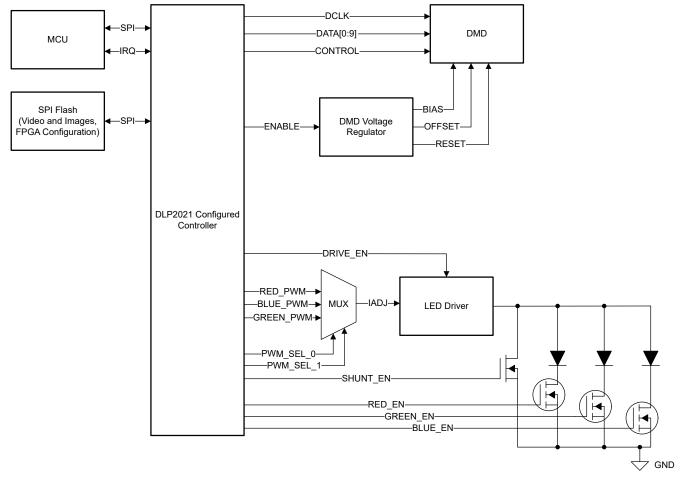
Figure 8-1. Dynamic Ground Projection System Block Diagram
