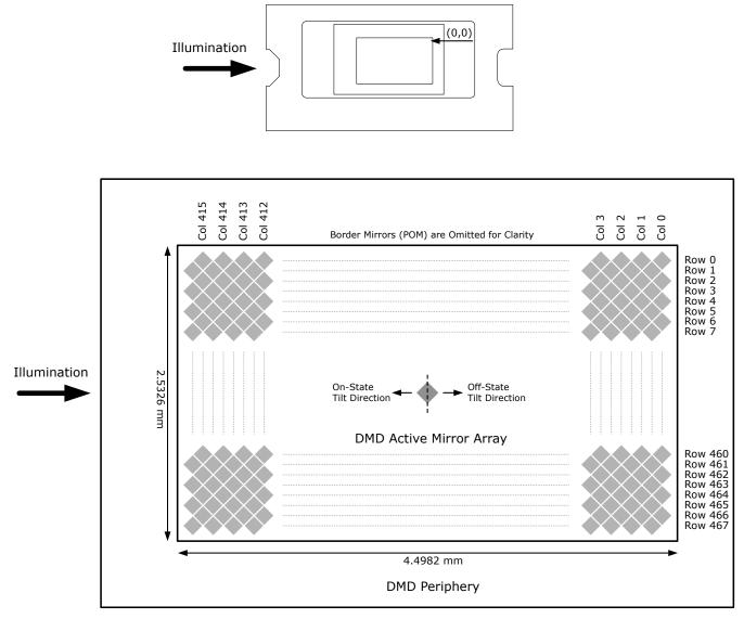
Figure 6-5. Micromirror Array Physical Characteristics
