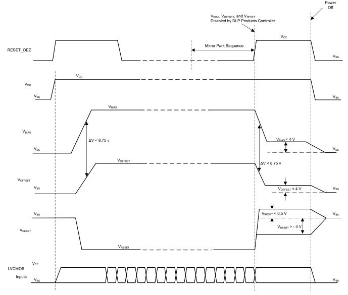
A.  $\pm 8.75$ -V delta,  $\Delta V$ , shall be considered the max operating delta between V<sub>BIAS</sub> and V<sub>OFFSET</sub>. Customers may find that the most reliable way to ensure this is to power V<sub>OFFSET</sub> prior to V<sub>BIAS</sub> during power up and to remove V<sub>BIAS</sub> prior to V<sub>OFFSET</sub> during power down.
