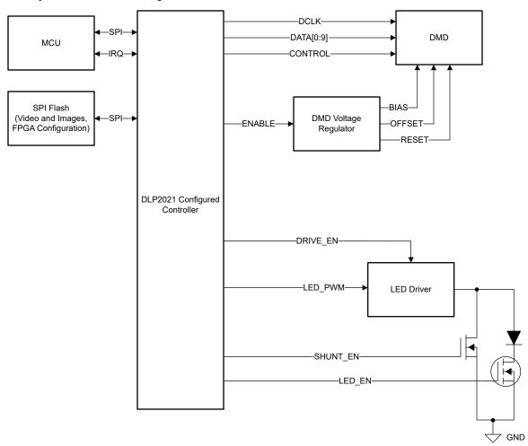
Figure 8-2. Dynamic Ground Projection System Block Diagram - Single Color
