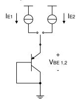
Figure 7-2. Temperature Measurement Theory
