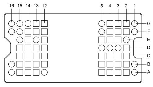
Figure 5-1. FQU Package 64-Pin LGA Bottom View
