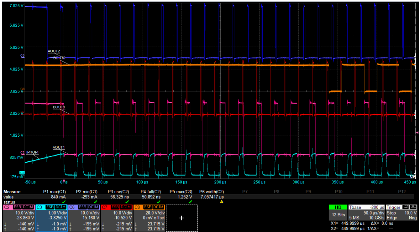
Figure 7-2. Driving four loads simultaneously
