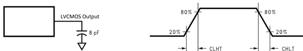
Figure 2. LVCMOS Output Load and Transition Times
