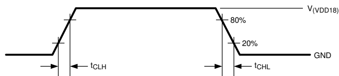
Figure 5-1. LVC MOS Transition Times
