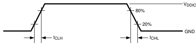
Figure 4-1. LVCMOS Transition Times
