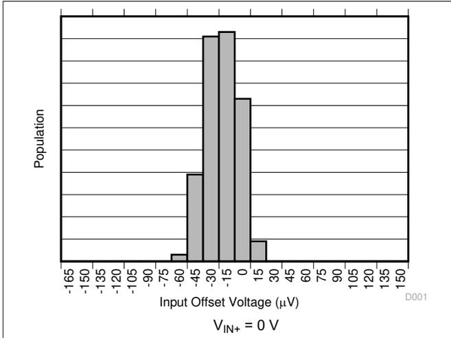
Figure 7-1. Input Offset Voltage Production Distribution A1
