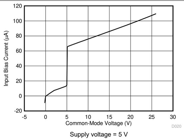
**Figure 7-20. Input Bias Current vs. Common-Mode Voltage**
