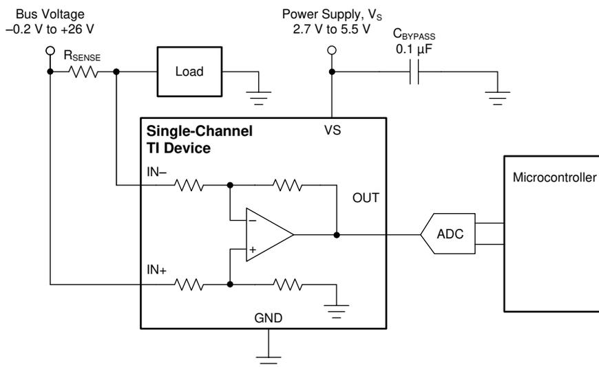
NOTE: For best measurement accuracy, connect analog-to-digital converter (ADC) reference or microcontroller ground as closely as possible to the INAx180-Q1 GND pin, and add an RC filter between the output of the INAx180-Q1 and the ADC. See [Closed-Loop Analysis of Load-Induced Amplifier Stability Issues Using Z<sub>OUT</sub>](#) for more details.
