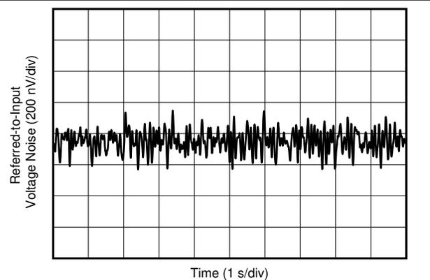
Figure 7-30. 0.1-Hz to 10-Hz Voltage Noise (Referred-to-Input)
