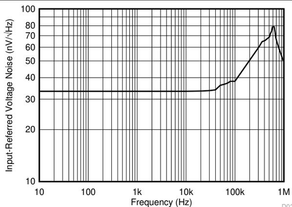
Figure 7-29. Input-Referred Voltage Noise vs. Frequency (A3 Devices)
