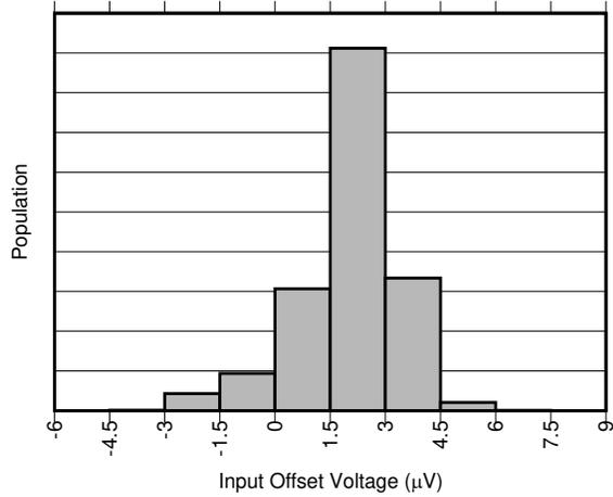
**Figure 6-5. Input Offset Production Distribution, A5 Devices**
