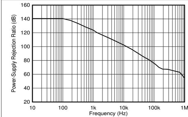
Figure 6-13. Power-Supply Rejection Ratio vs. Frequency
