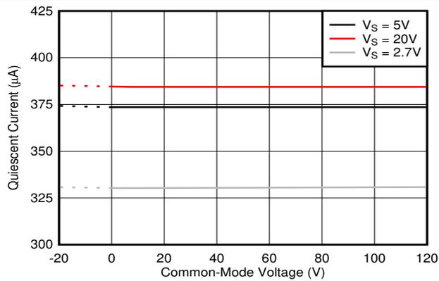
Figure 6-37. Quiescent Current vs. Common-Mode Voltage, INA2290
