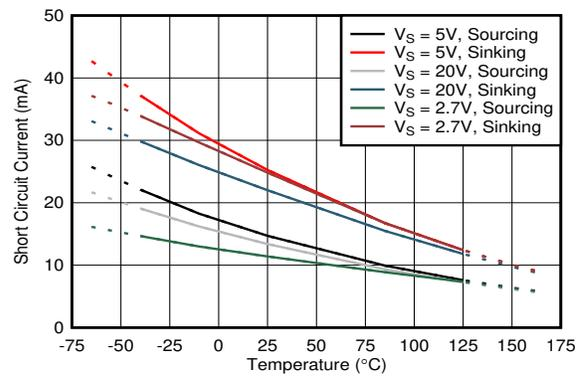
**Figure 6-22. Short-Circuit Current vs. Temperature**
