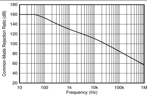
**Figure 6-9. Common-Mode Rejection Ratio vs. Frequency**
