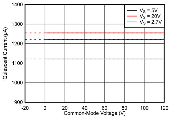
Figure 6-39. Quiescent Current vs. Common-Mode Voltage, INA4290
