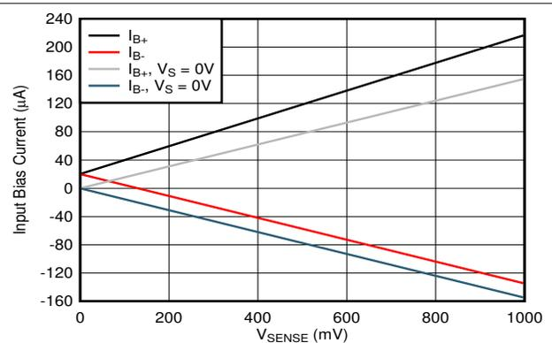
Figure 6-16. Input Bias Current vs.  $V_{\text{SENSE}}$
