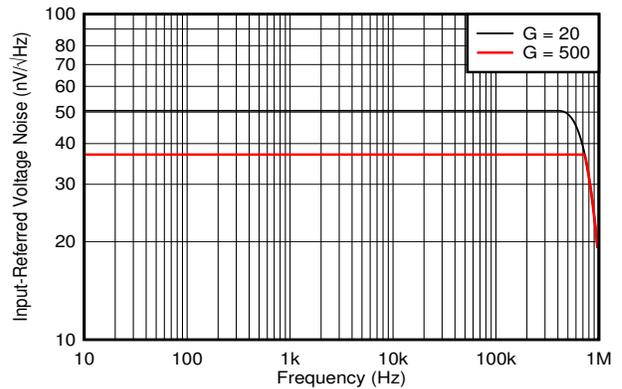
**Figure 6-26. Input-Referred Noise vs. Frequency**
