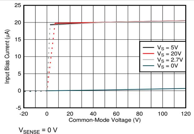
Figure 6-14. Input Bias Current vs. Common-Mode Voltage
