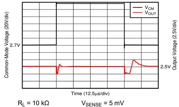
Figure 6-40. Common-Mode Voltage Fast Transient Pulse, A5 Devices
