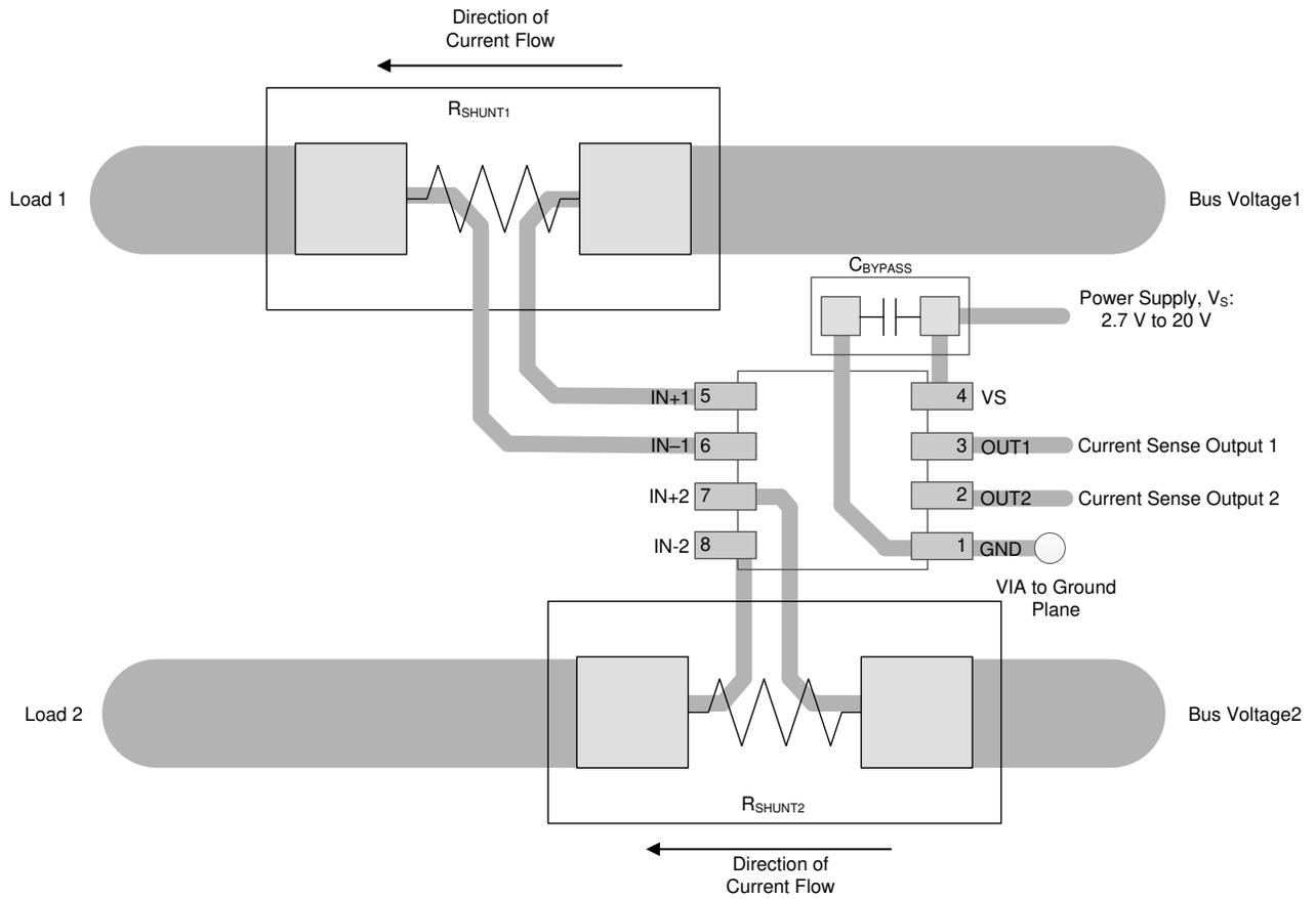
**Figure 10-2. Recommended Layout for the INA2290**
