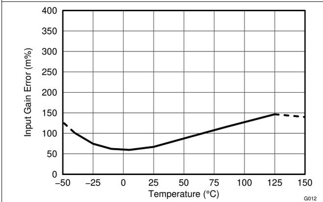
Figure 6-11. Bus Input Gain Error vs. Temperature
