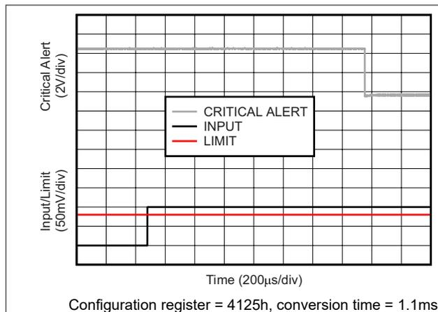
**Figure 8-2. Critical Alert Response for 1.1ms Conversion Time**
