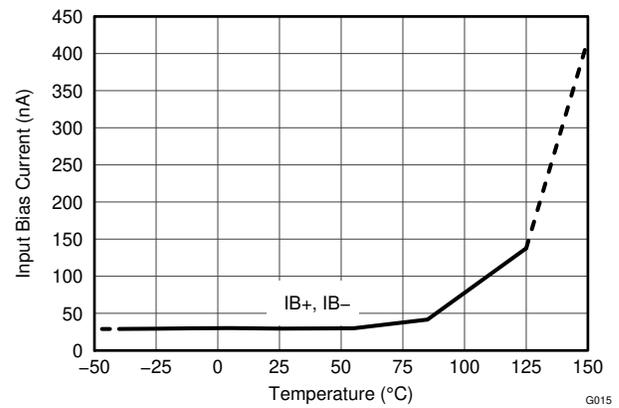
**Figure 6-14. Input Bias Current vs. Temperature (Shutdown)**
