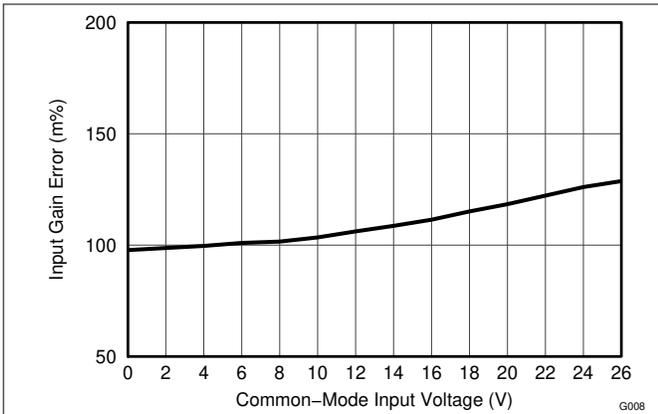
Figure 6-7. Shunt Input Gain Error vs. Common-Mode Voltage
