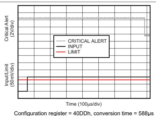
**Figure 8-3. Critical Alert Response for 588 $\mu$ s Conversion Time**
