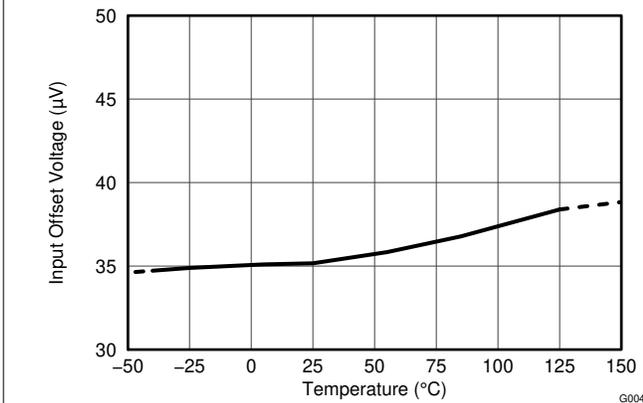
**Figure 6-3. Shunt Input Offset Voltage vs. Temperature**
