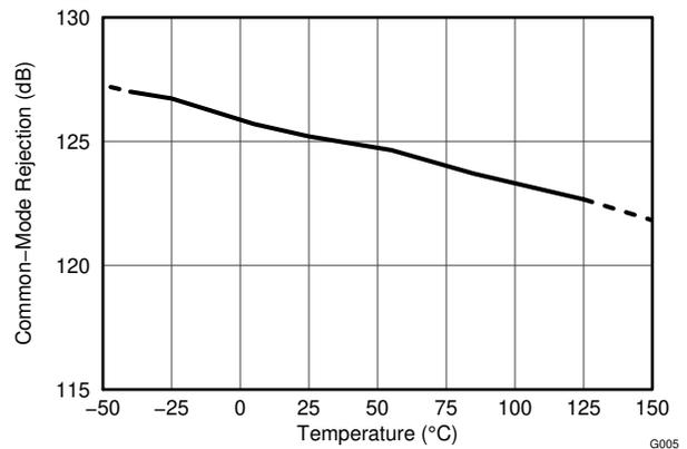
**Figure 6-4. Shunt Input Common-Mode Rejection Ratio vs. Temperature**
