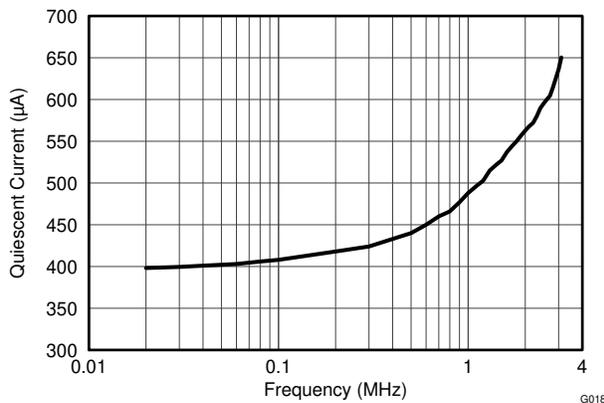
**Figure 6-17. Active  $I_Q$  vs.  $I^2\text{C}$  Clock Frequency**
