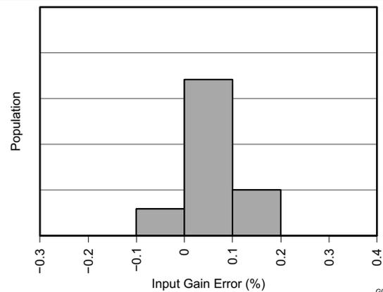
Figure 6-10. Bus Input Gain Error Production Distribution
