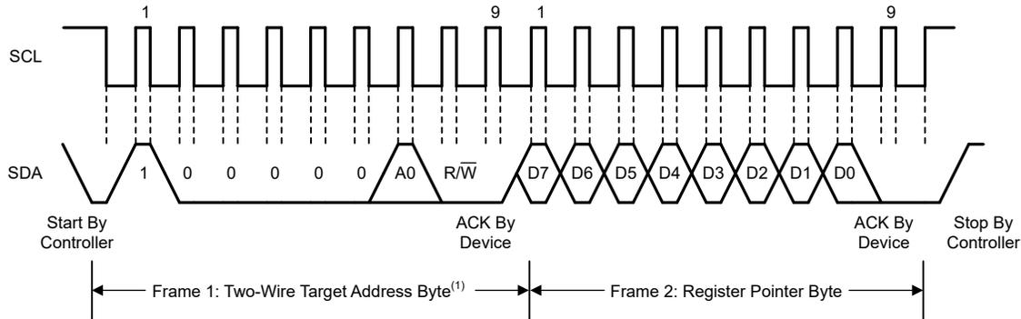
A. The value of the Target Address Byte is determined by the A0 pin setting; see Table 7-1.
