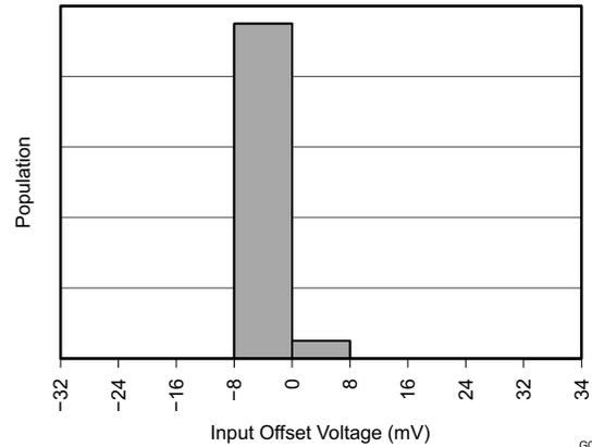
Figure 6-8. Bus Input Offset Voltage Production Distribution
