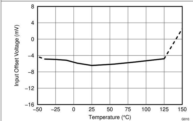
Figure 6-9. Bus Input Offset Voltage vs. Temperature
