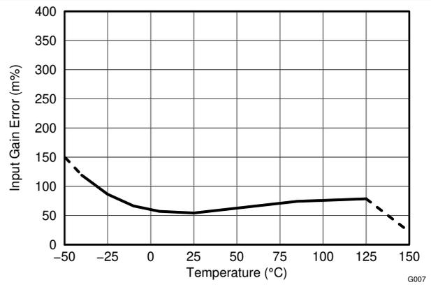
**Figure 6-6. Shunt Input Gain Error vs. Temperature**
