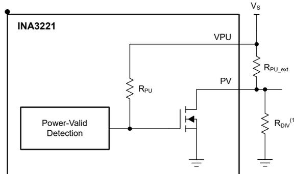
A.  $R_{DIV}$  can be used to level-shift the PV output high.
