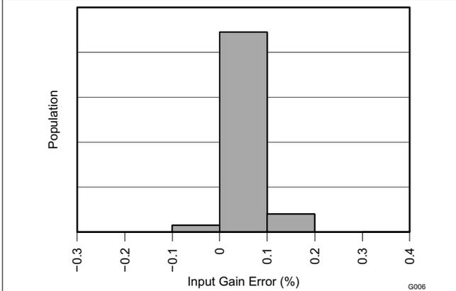
**Figure 6-5. Shunt Input Gain Error Production Distribution**
