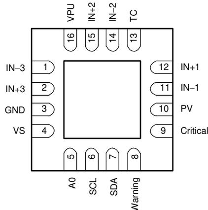
**Figure 5-1. RGV Package 16-Pin VQFN Top View**
