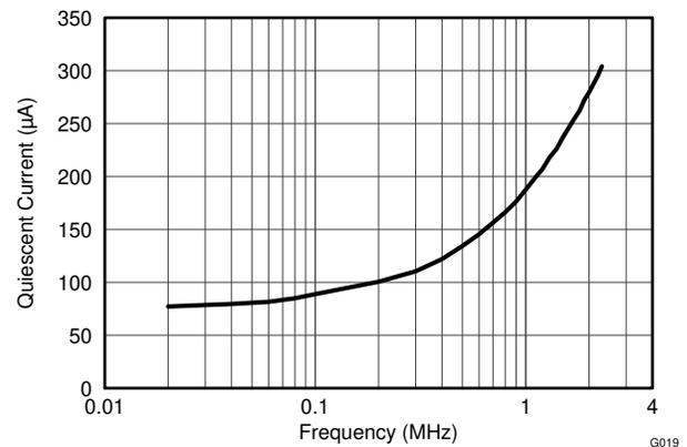
**Figure 6-18. Shutdown  $I_Q$  vs.  $I^2\text{C}$  Clock Frequency**
