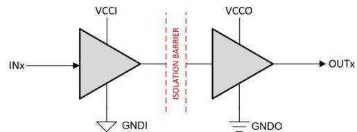
$V_{CCI}$  and  $GNDI$  are supply and ground connections respectively for the input channels.
