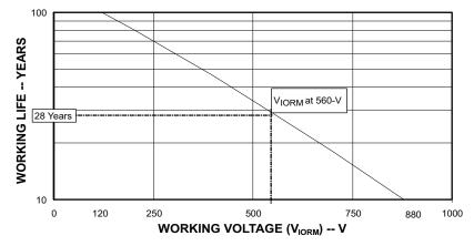
Figure 10. Time-Dependant Dielectric Breakdown Testing Results
