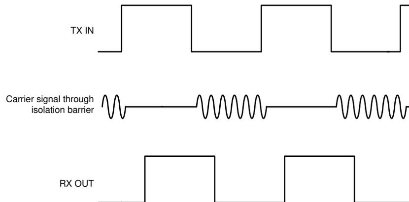
**Figure 24-2. On-Off Keying (OOK) Based Modulation Scheme**
