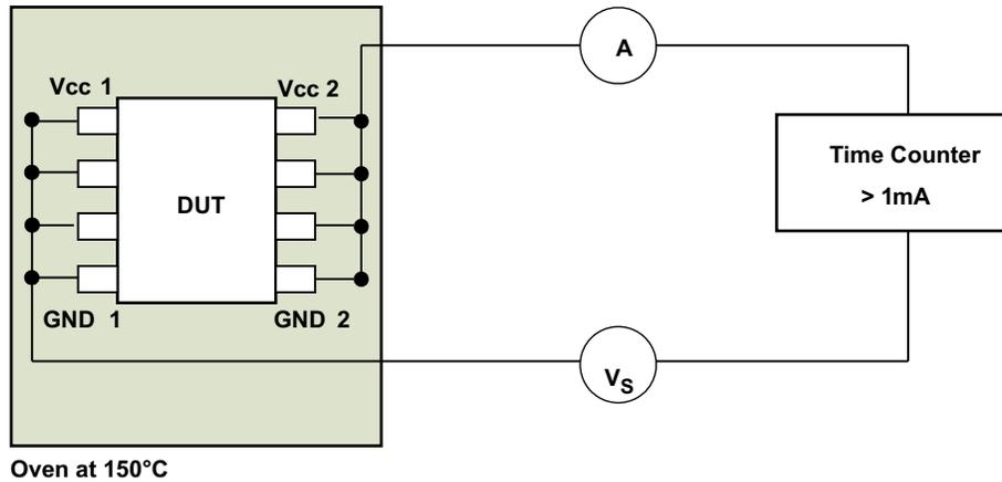
Figure 25-4. Test Setup for Insulation Lifetime Measurement
