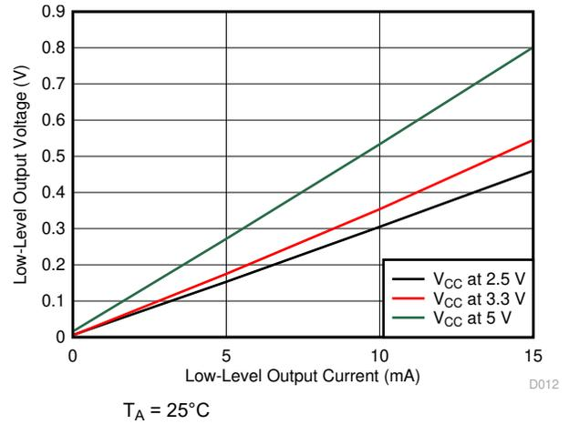
**Figure 5-12. Low-Level Output Voltage vs Low-Level Output Current**
