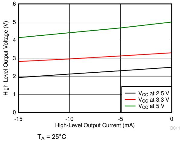
**Figure 5-11. High-Level Output Voltage vs High-level Output Current**
