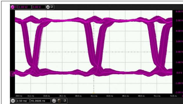
**Figure 8-3. Eye Diagram at 100 Mbps PRBS 2<sup>16</sup> – 1 Data, 5 V and 25°C**
