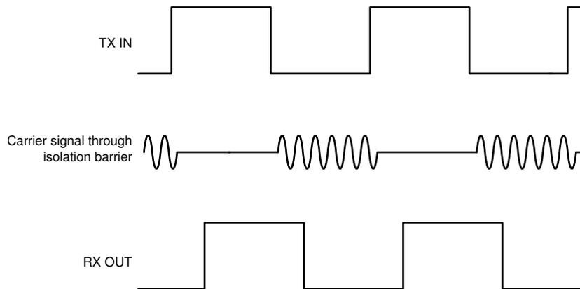
**Figure 7-2. ON-OFF Keying (OOK) Based Modulation Scheme**
