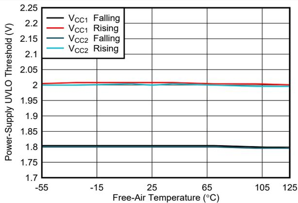
**Figure 5-15. Power Supply Undervoltage Threshold vs Free-Air Temperature**
