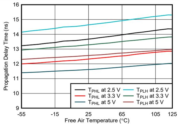
**Figure 5-16. Propagation Delay Time vs Free-Air Temperature**
