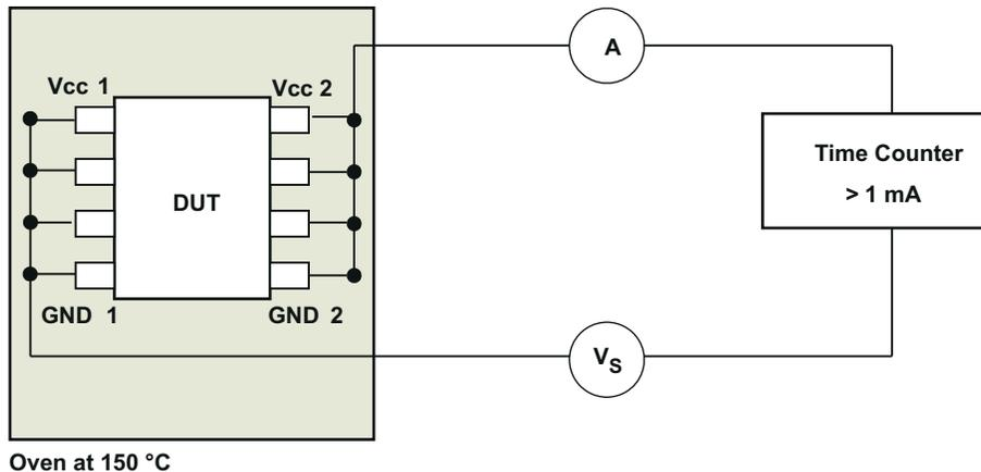
Figure 8-6. Test Setup for Insulation Lifetime Measurement
