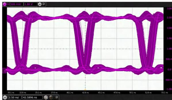
**Figure 8-5. Eye Diagram at 100 Mbps PRBS 2<sup>16</sup> – 1 Data, 2.5 V and 25°C**
