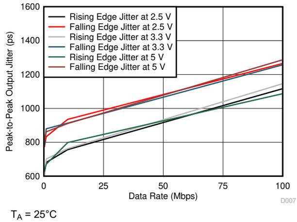
**Figure 5-17. Peak-to-Peak Output Jitter vs Data Rate**
