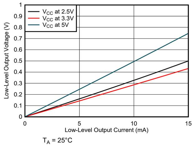
**Figure 5-14. Low-Level Output Voltage vs Low-Level Output Current**
