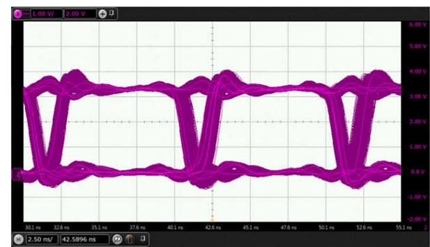
**Figure 8-4. Eye Diagram at 100 Mbps PRBS 2<sup>16</sup> – 1 Data, 3.3 V and 25°C**
