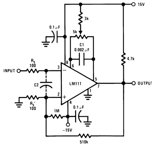
Pin connections shown are for LM111H in the LMC0008C hermetic package
