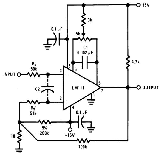
Figure 22. Positive Feedback with High Source Resistance
