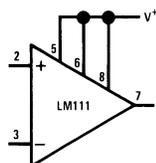
**Note:** Increases typical common mode slew from 7.0V/ $\mu$ s to 18V/ $\mu$ s.
