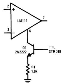
**Note:** Do Not Ground Strobe Pin. Output is turned off when current is pulled from Strobe Pin.
