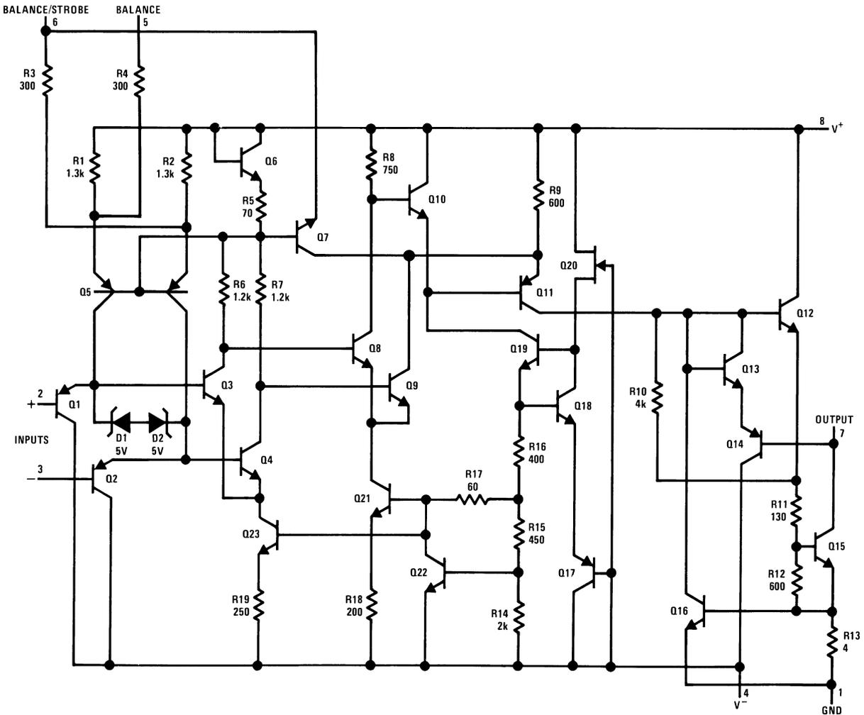
Note: Pin connections shown on schematic diagram are for LMC0008C package.
