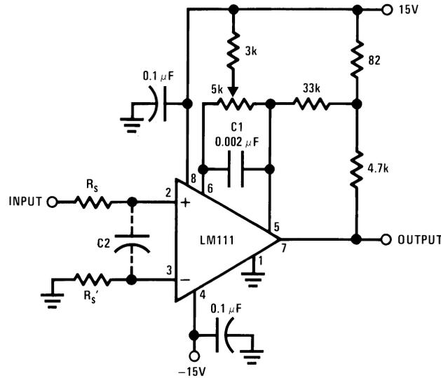
Pin connections shown are for LM111H in the LMC0008C hermetic package
