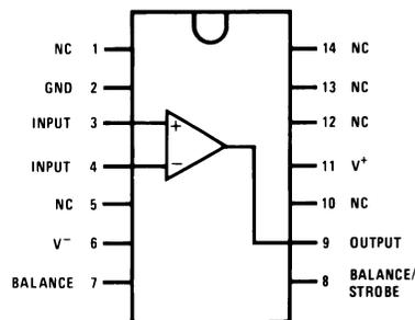
**Figure 3. Dual-In-Line Package
