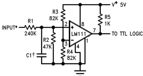
\*Values shown are for a 0 to 30V logic swing and a 15V threshold.
