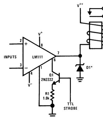
\*Absorbs inductive kickback of relay and protects IC from severe voltage transients on V<sup>++</sup> line.
