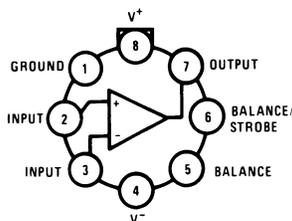
Note: Pin 4 connected to case
