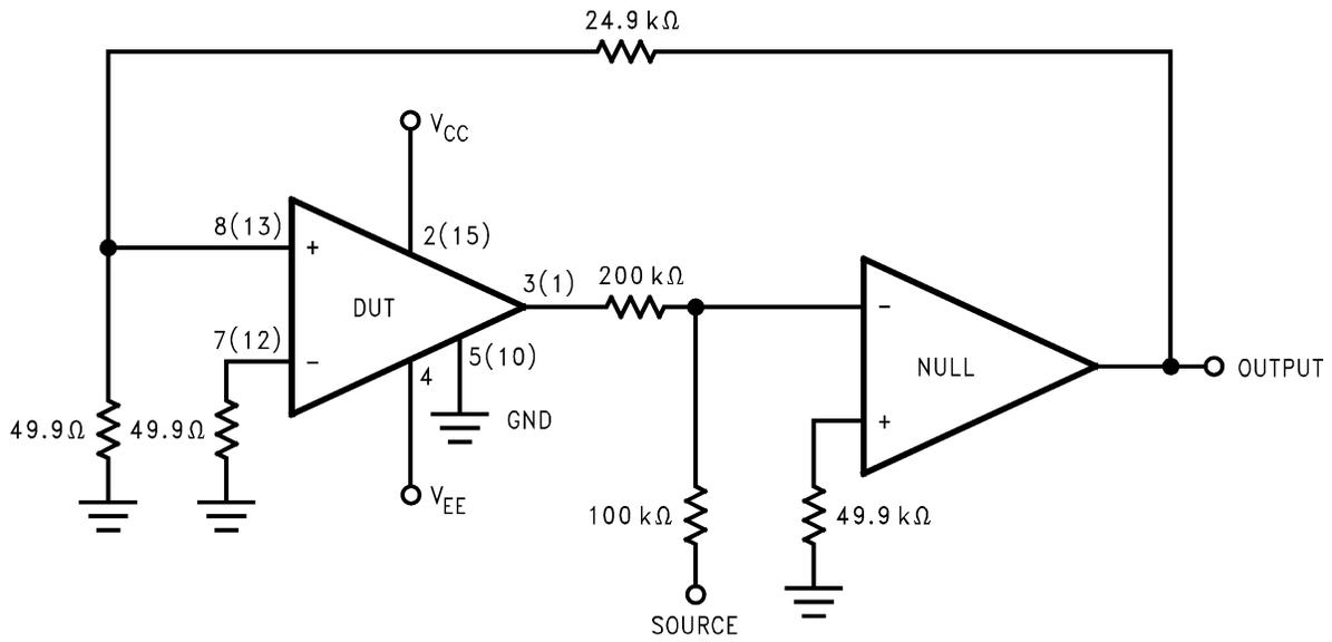
**Test Circuit #2 (AC Electrical Test Circuit)**
