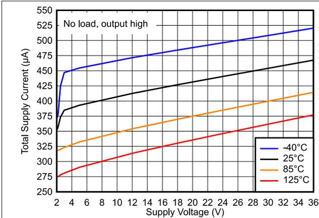
Figure 5-1. Total Supply Current vs. Supply Voltage
