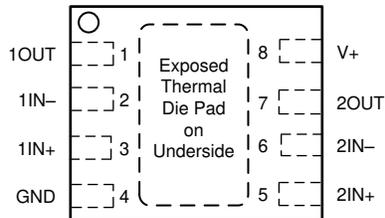
Connect thermal pad directly to GND pin.
