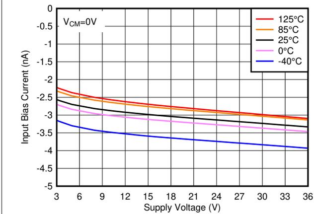
Figure 5-15. Input Bias Current vs. Supply Voltage
