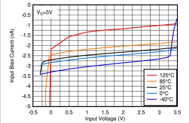
Figure 5-16. Input Bias Current vs. Input Voltage at 5V
