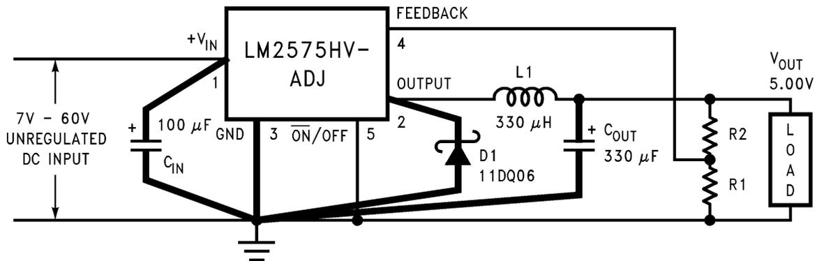
$$V_{OUT} = V_{REF} \left( 1 + \frac{R2}{R1} \right)$$
