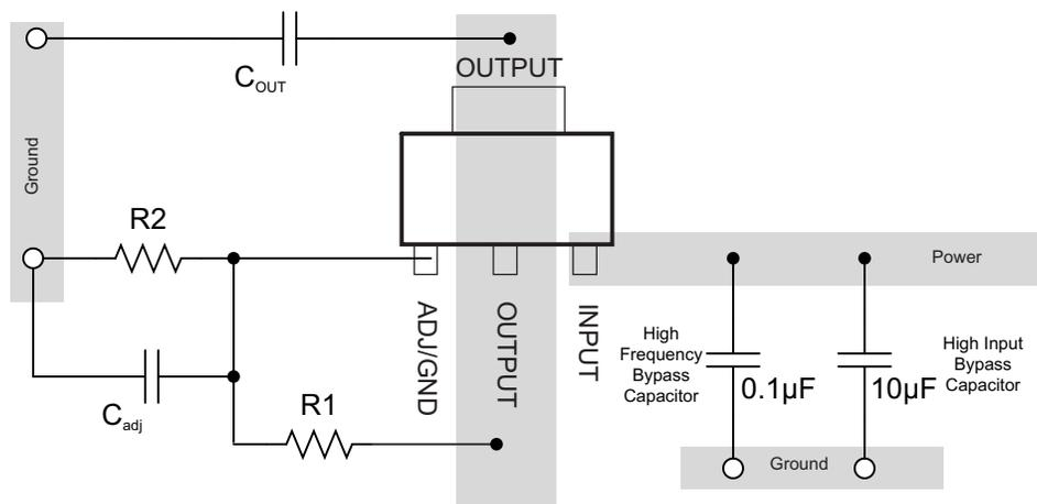
Figure 7-11. Layout Diagram
