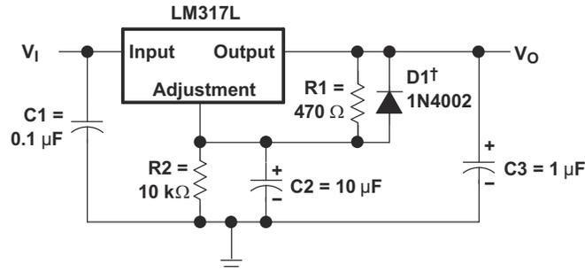
Figure 7-3. Regulator Circuit With Improved Ripple Rejection
