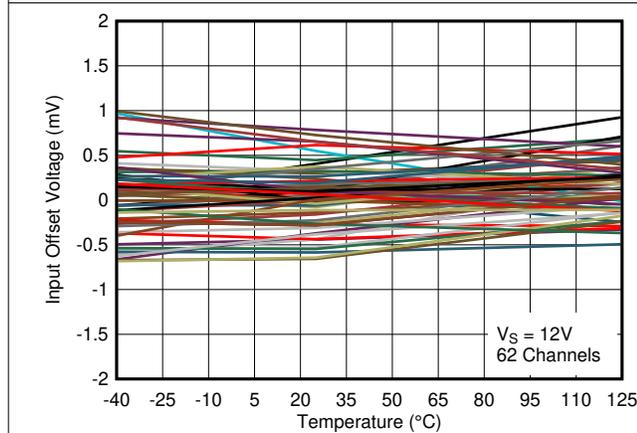
Figure 6-9. Input Offset Voltage vs. Temperature at 12V
