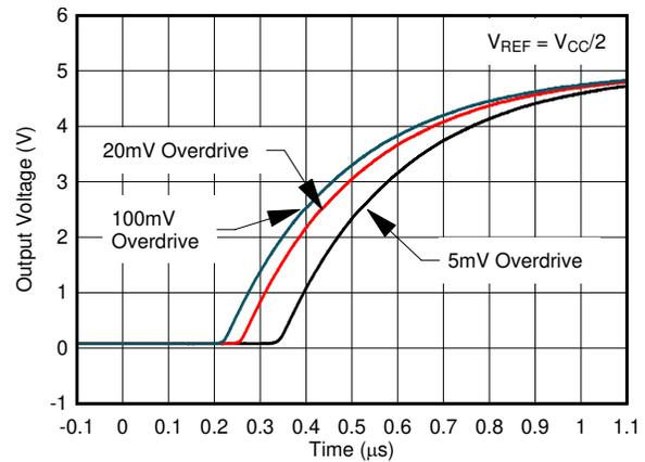
**Figure 6-32. Response Time for Various Overdrives, Low-to-High Transition**
