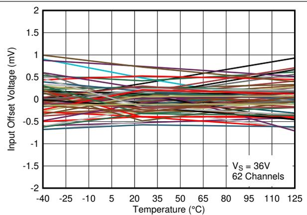
Figure 6-10. Input Offset Voltage vs. Temperature at 36V
