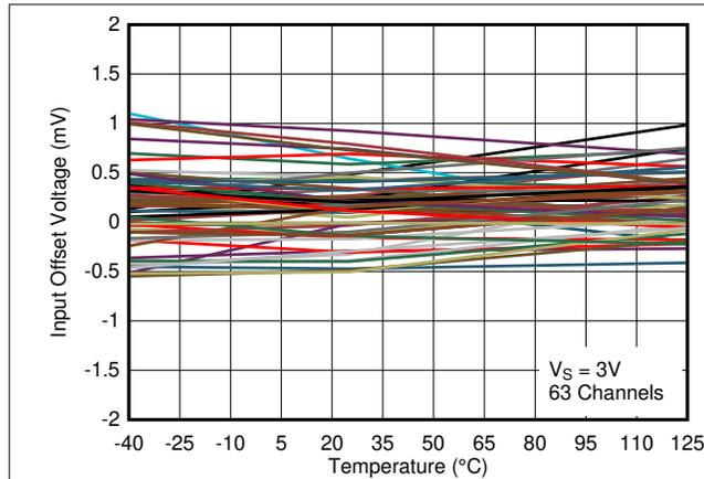
Figure 6-7. Input Offset Voltage vs. Temperature at 3V
