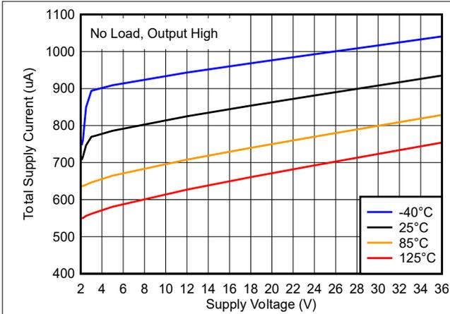
Figure 6-1. Total Supply Current vs. Supply Voltage
