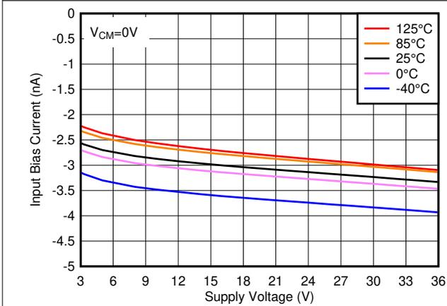
Figure 6-15. Input Bias Current vs. Supply Voltage
