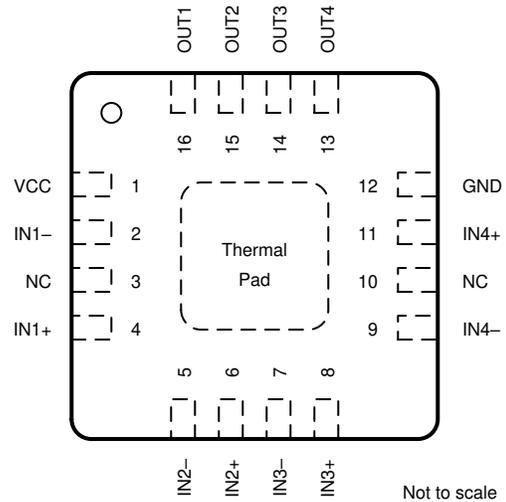
NOTE: Connect exposed thermal pad directly to GND pin.
