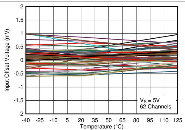
Figure 6-8. Input Offset Voltage vs. Temperature at 5V
