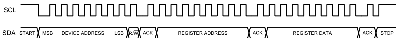
Figure 26. Example I 2 C Write Cycle
