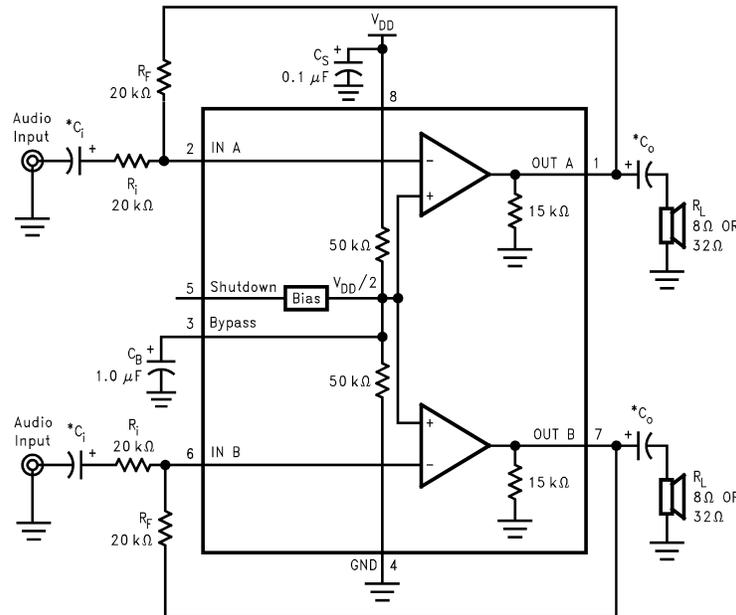
\*Refer to [Application Information](#) for information concerning proper selection of the input and output coupling capacitors.
