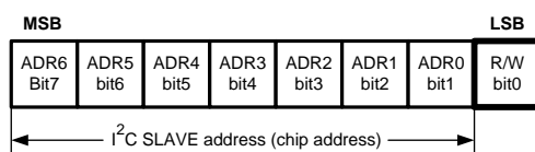
Figure 5. I 2 C Chip Address
