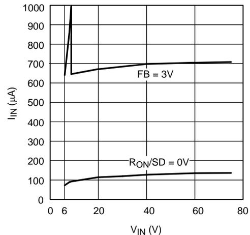
Figure 7.  $I_{IN}$  vs  $V_{IN}$
