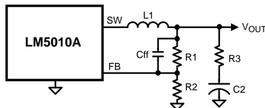
**Figure 14. Low Output Ripple Using a Feed-Forward Capacitor**
