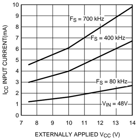
Figure 4.  $I_{CC}$  vs Externally Applied  $V_{CC}$
