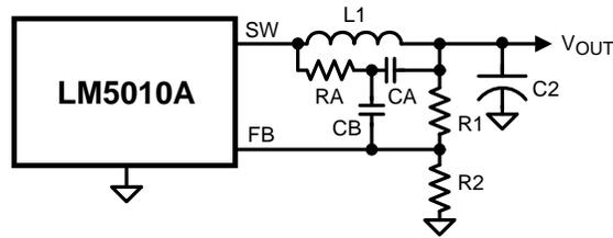
Figure 15. Low Output Ripple Using Ripple Injection
