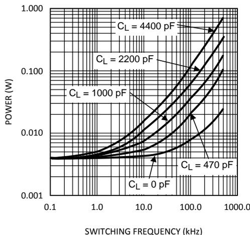
**Figure 20. Gate Driver Power Dissipation (LO + HO)**
