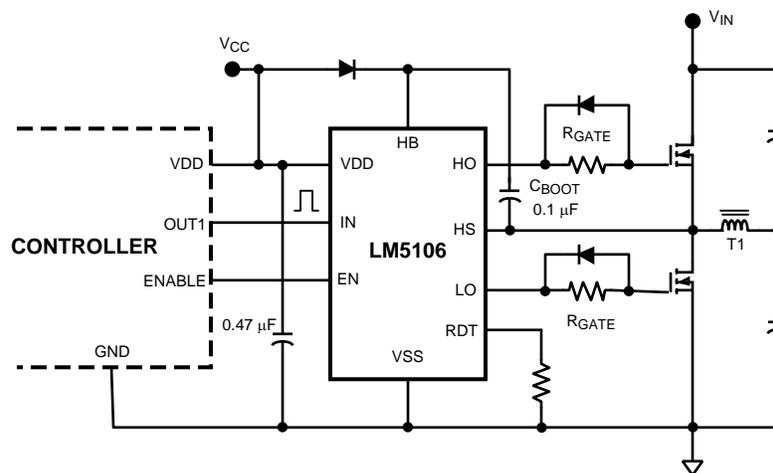
Figure 17. LM5106 Driving MOSFETs Connected in Half-Bridge Configuration
