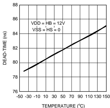
Figure 15. Dead-Time vs Temperature (RT = 10k)
