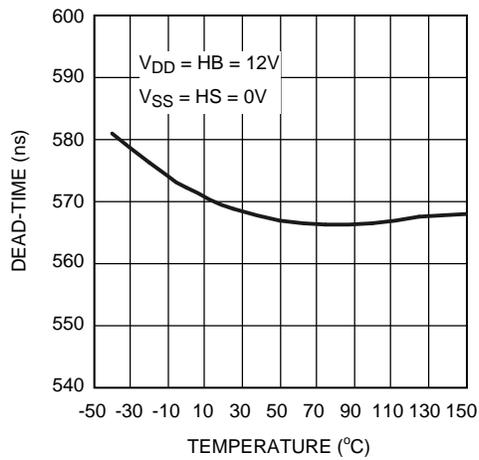
**Figure 16. Dead-Time vs Temperature (RT = 100k)**
