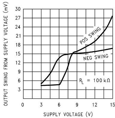
**Figure 5-9. Output Voltage Swing vs Supply Voltage**
