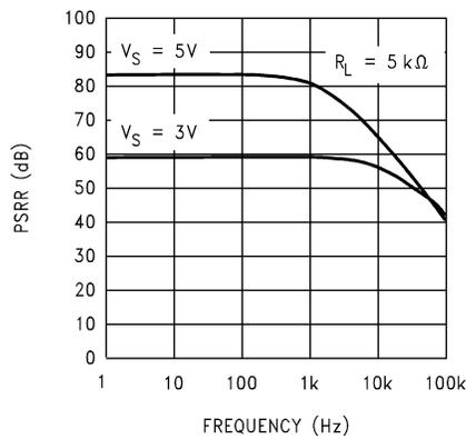
Figure 5-13. Positive PSRR vs Frequency
