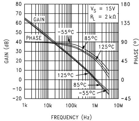
Figure 5-20. Open Loop Frequency Response vs Temperature
