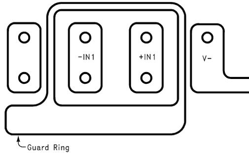
**Figure 6-15. Examples of Guard Ring in PCB Layout**
