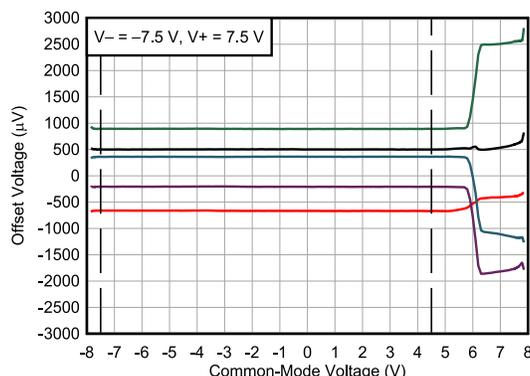
**Figure 6-2. Input Offset Voltage vs Common-Mode Voltage**
