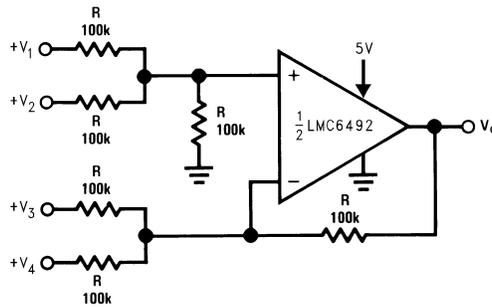
Where:  $V_0 = V_1 + V_2 - V_3 - V_4$
