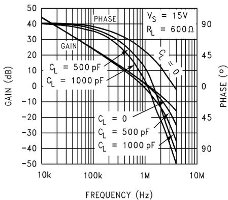
Figure 5-23. Gain and Phase vs Capacitive Load
