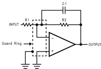
**Figure 6-16. Inverting Amplifier**
