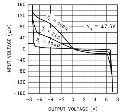
Figure 5-16. Input Voltage vs Output Voltage
