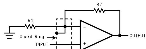
**Figure 6-17. Noninverting Amplifier**
