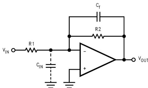
**Figure 6-5. Canceling the Effect of Input Capacitance**
