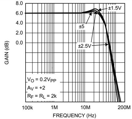
Figure 8. Closed Loop Small Signal Frequency Response for Various Supplies
