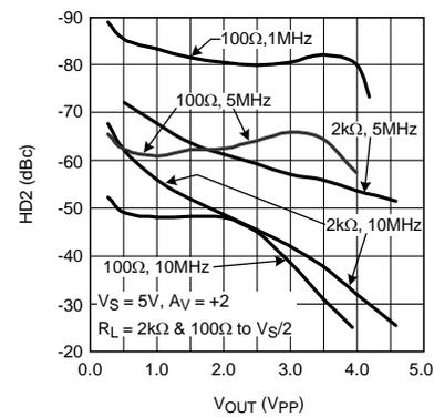
Figure 18. HD2 vs. Output Swing
