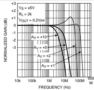
Figure 2. Closed Loop Gain vs. Frequency for Various Gain
