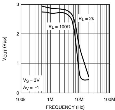
Figure 11.  $V_{OUT}$  ( $V_{PP}$ ) for THD < 0.5%
