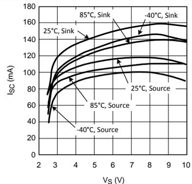
Figure 28. Short Circuit Current (to  $V_S/2$ ) vs.  $V_S$
