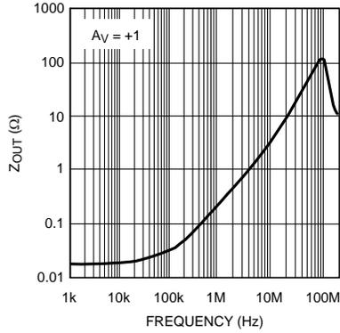
Figure 31. Closed Loop Output Impedance vs. Frequency  $A_V = +1$
