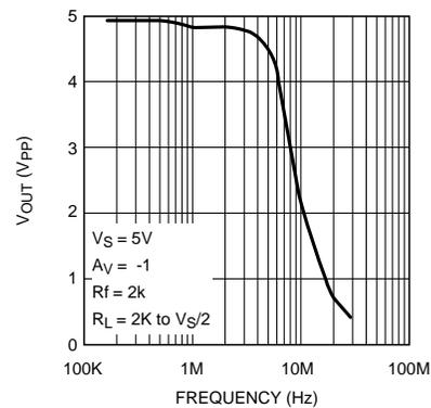
Figure 12.  $V_{OUT}$  ( $V_{PP}$ ) for THD < 0.5%
