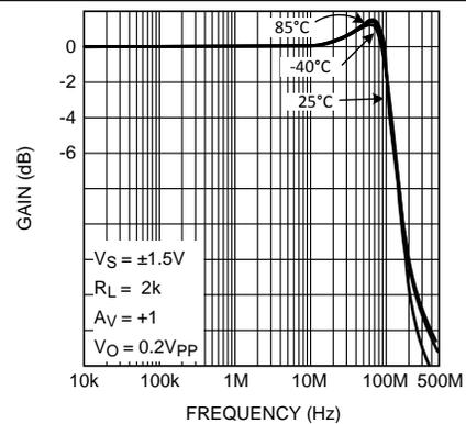
Figure 4. Closed Loop Frequency Response for Various Temperature
