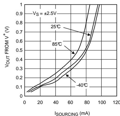
Figure 30. Output Sourcing Saturation Voltage vs.  $I_{OUT}$
