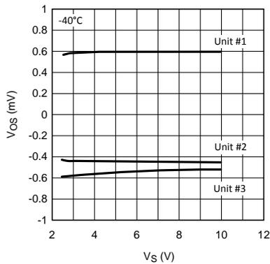
**Figure 37.  $V_{OS}$  vs.  $V_S$  (for 3 Representative Units)**
