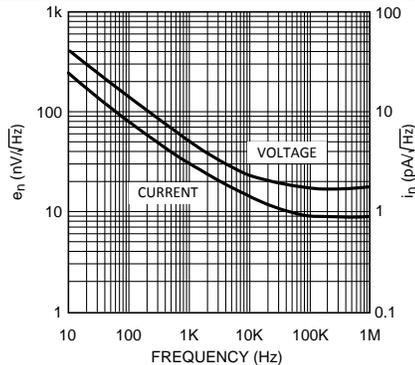
Figure 22. Input Noise vs. Frequency
