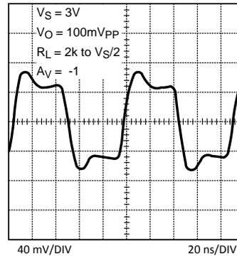
Figure 44. Small Signal Step Response
