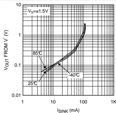
Figure 24.  $V_{OUT}$  from  $V^-$  vs.  $I_{SINK}$
