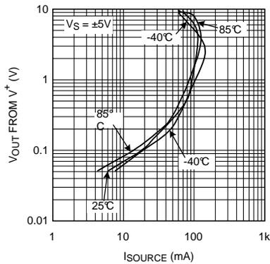
Figure 25.  $V_{OUT}$  from  $V^+$  vs.  $I_{SOURCE}$
