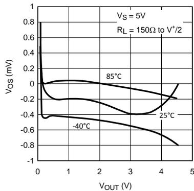
Figure 35.  $V_{OS}$  vs.  $V_{OUT}$  (Typical Unit)
