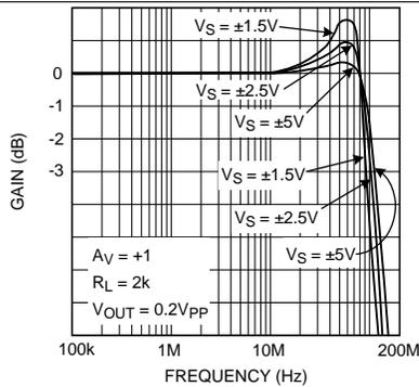
Figure 1. Closed Loop Frequency Response for Various Supplies
