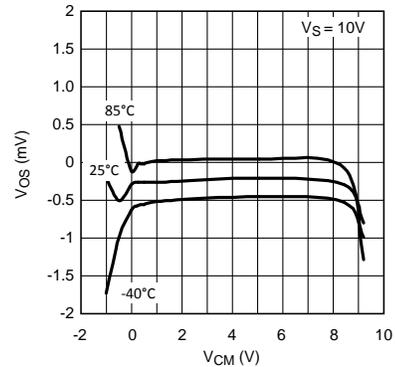
Figure 36.  $V_{OS}$  vs.  $V_{CM}$  (Typical Unit)
