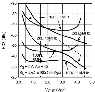
Figure 19. HD3 vs. Output Swing
