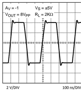
**Figure 53. Large Signal Step Response**
