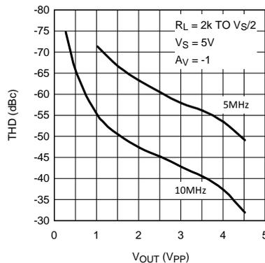
Figure 20. THD (dBc) vs. Output Swing
