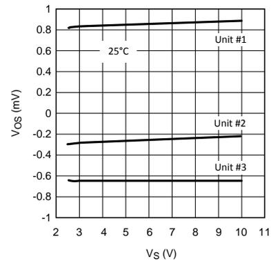
**Figure 38.  $V_{OS}$  vs.  $V_S$  (for 3 Representative Units)**
