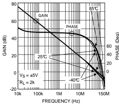
Figure 15. Open Loop Gain/Phase for Various Temperature
