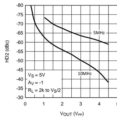
Figure 16. HD2 (dBc) vs. Output Swing
