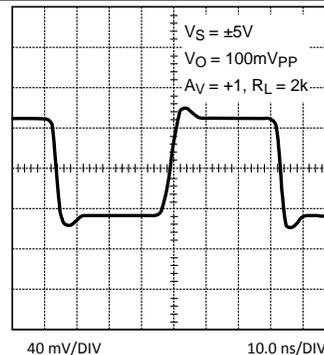
Figure 48. Small Signal Step Response
