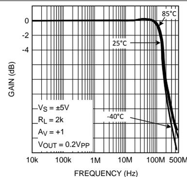
Figure 6. Closed Loop Frequency Response for Various Temperature
