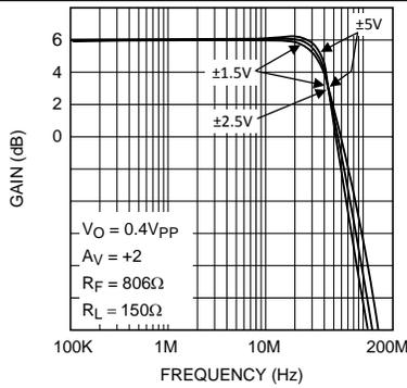
Figure 9. Closed Loop Frequency Response for Various Supplies
