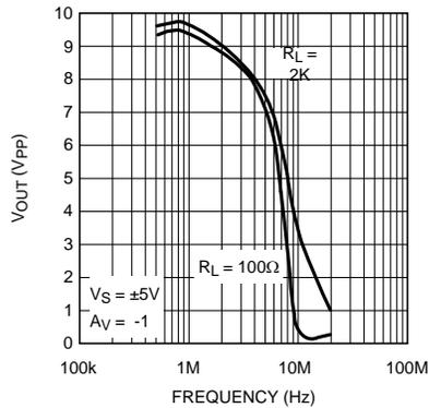
Figure 13.  $V_{OUT}$  (V<sub>PP</sub>) for THD < 0.5%
