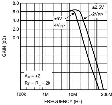
Figure 7. Large Signal Frequency Response
