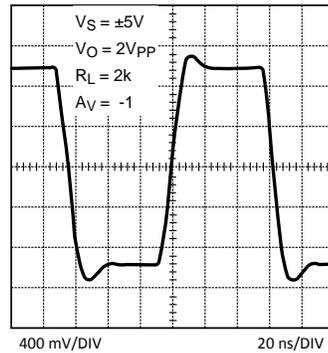
**Figure 52. Large Signal Step Response**
