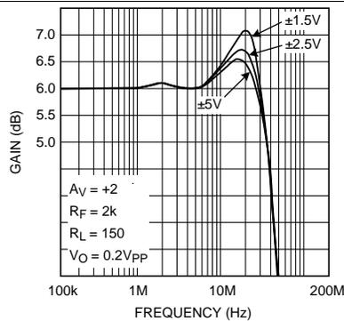
Figure 5. Closed Loop Gain vs. Frequency for Various Supplies
