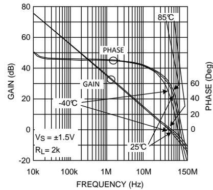
Figure 14. Open Loop Gain/Phase for Various Temperature
