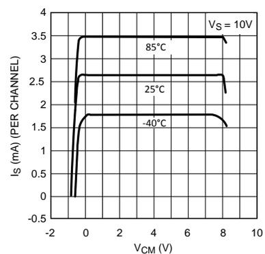
**Figure 42.  $I_S$  vs.  $V_{CM}$**
