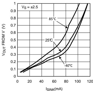
Figure 29. Output Sinking Saturation Voltage vs.  $I_{OUT}$
