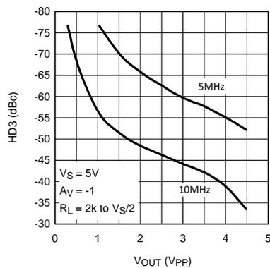
Figure 17. HD3 (dBc) vs. Output Swing
