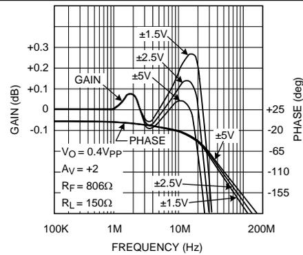
Figure 10.  $\pm 0.1\text{dB}$  Gain Flatness for Various Supplies
