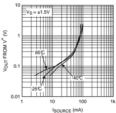
Figure 23.  $V_{OUT}$  from  $V^+$  vs.  $I_{SOURCE}$
