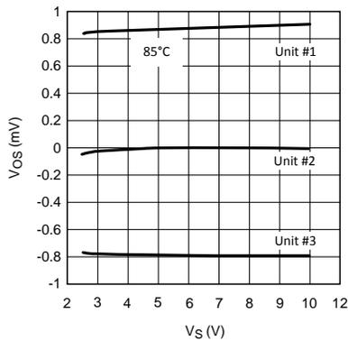
**Figure 39.  $V_{OS}$  vs.  $V_S$  (for 3 Representative Units)**
