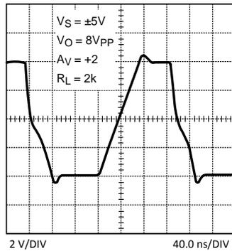
**Figure 51. Large Signal Step Response**
