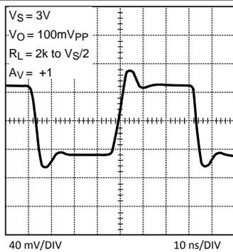
Figure 47. Small Signal Step Response
