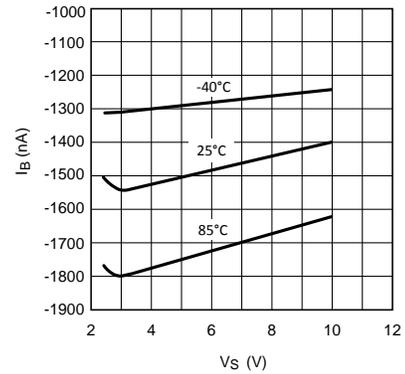
**Figure 40.  $I_B$  vs.  $V_S$**
