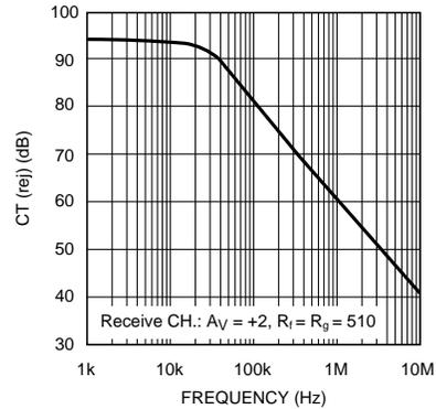
Figure 34. Crosstalk Rejection vs. Frequency (Output to Output)
