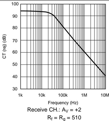
Figure 21. Crosstalk Rejection vs. Frequency (Output to Output, LMH6646)
