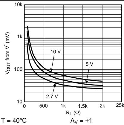
Figure 15. Output Swing from  $V^-$  vs.  $R_L$  (Tied to  $V_S/2$ )
