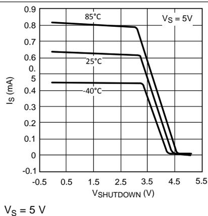
Figure 35.  $I_S$  vs.  $V_{SHUTDOWN}$  (LMH6647)
