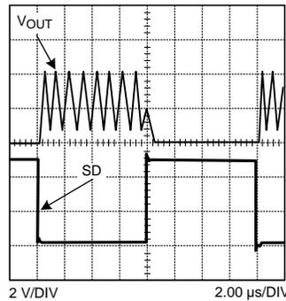
Figure 44. Output Held Low by Active Pull-Down Circuit
