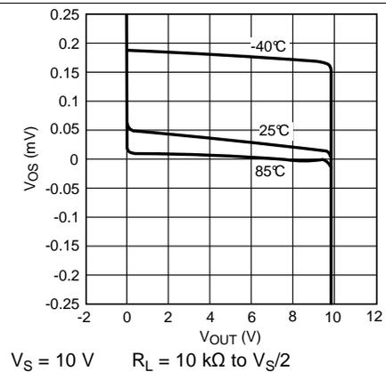
Figure 24.  $V_{OS}$  vs.  $V_{OUT}$  (a Typical Unit)
