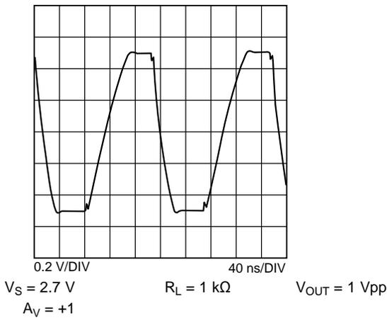
Figure 39. Large Signal Step Response
