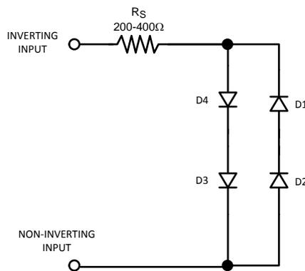
**Figure 42. LMH6647 Equivalent Input in Shutdown Mode**
