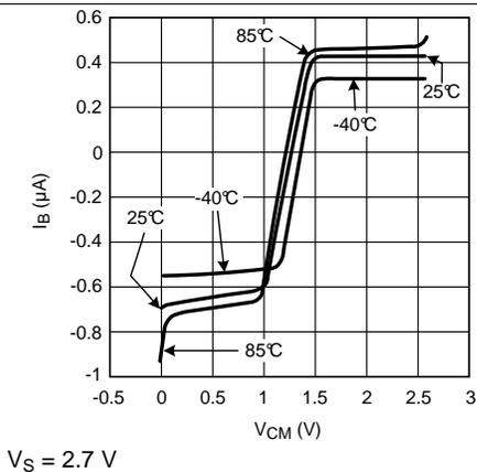
Figure 29.  $I_B$  vs.  $V_{CM}$
