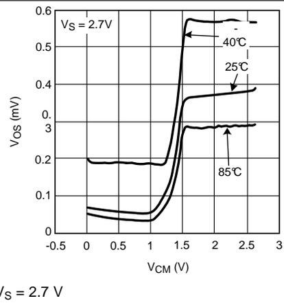
Figure 26.  $V_{OS}$  vs.  $V_{CM}$  (a Typical Unit)
