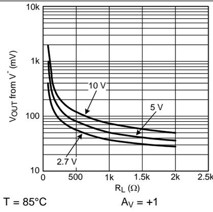
Figure 16. Output Swing from  $V^-$  vs.  $R_L$  (Tied to  $V_S/2$ )
