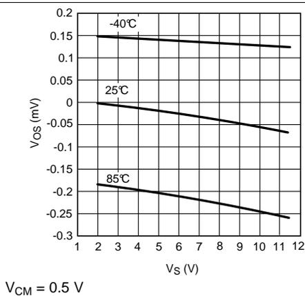
Figure 23.  $V_{OS}$  vs.  $V_S$  (a Typical Unit)
