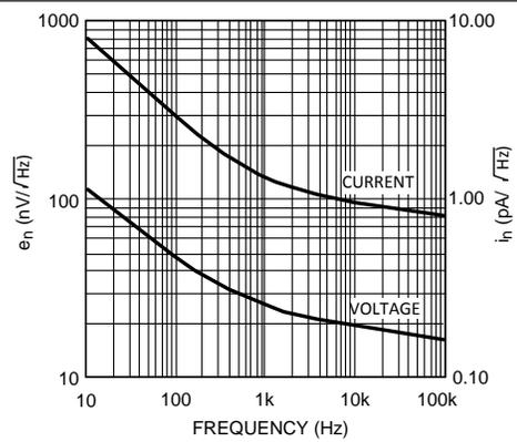
Figure 8. Noise vs. Frequency
