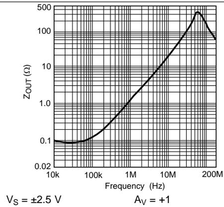
Figure 18.  $Z_{OUT}$  vs. Frequency
