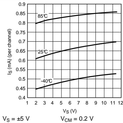
Figure 33.  $I_S$  (mA) vs.  $V_S$ (V)
