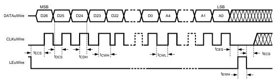
Figure 8. MICROWIRE Input Timing Diagram
