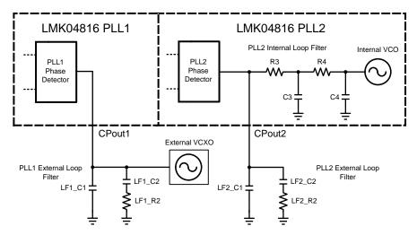
Figure 22. PLL1 and PLL2 Loop Filters
