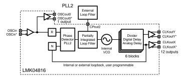
Figure 20. Simplified Functional Block Diagram for 0-Delay Single-Loop Mode
