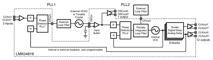
Figure 18. Simplified Functional Block Diagram for 0-Delay Dual-Loop Mode
