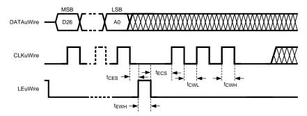
Figure 9. MICROWIRE Timing Diagram: Extra CLKuWire Pulses for R0 to R5
