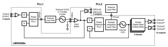
Figure 39. Simplified Functional Block Diagram for Dual-Loop Mode
