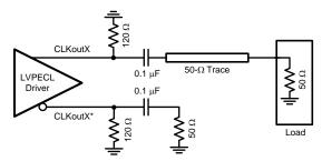
Figure 36. Single-Ended LVPECL Operation, AC Coupling
