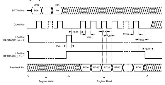
Figure 11. MICROWIRE Readback Timing Diagram
