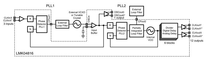
Figure 17. Simplified Functional Block Diagram for Dual-Loop Mode
