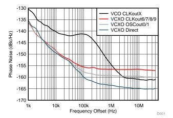
Figure 40. LVPECL Phase Noise, 122.88-MHz Illustration of Different Performance Depending on Signal Path
