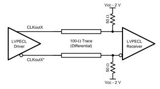
Figure 29. Differential LVPECL Operation, DC Coupling
