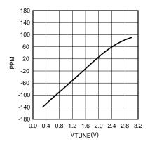
Figure 38. Example Tuning Curve, 20.48-MHz Crystal
