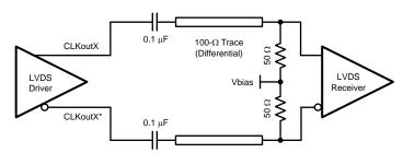
Figure 31. Differential LVDS Operation, AC Coupling, External Biasing at the Receiver
