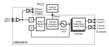
Figure 19. Simplified Functional Block Diagram for Single-Loop Mode
