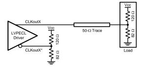
Figure 35. Single-Ended LVPECL Operation, DC Coupling, Thevenin Equivalent
