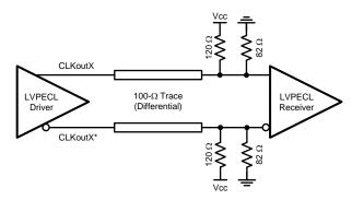
Figure 30. Differential LVPECL Operation, DC Coupling, Thevenin Equivalent
