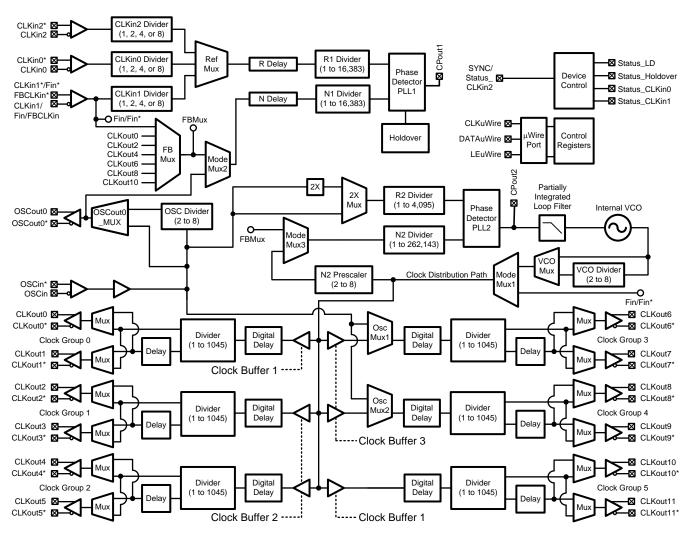
Figure 7. Detailed LMK04816 Block Diagram
