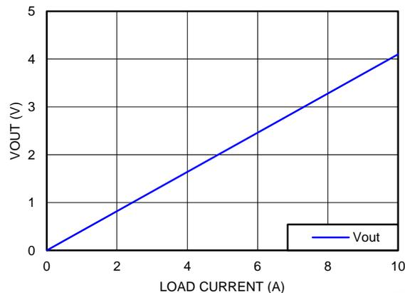
**Figure 28. Application Example Results using 8.2 mΩ Resistor**
