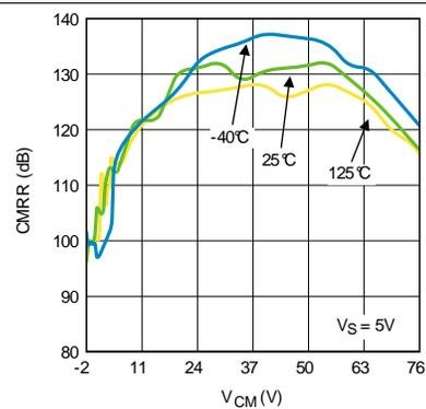
Figure 6. CMRR vs.  $V_{\text{CM}}$  (Gain 50 V/V)
