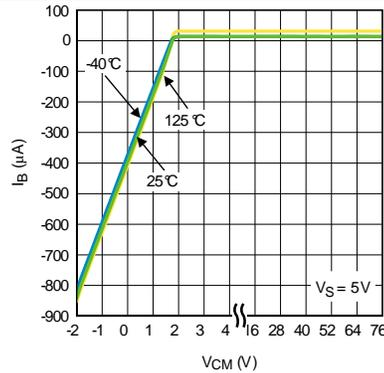
Figure 10.  $I_{\text{Bias}}$  vs.  $V_{\text{CM}}$
