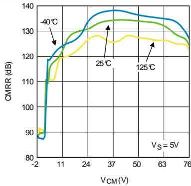
Figure 7. CMRR vs.  $V_{\text{CM}}$  (Gain 100 V/V)
