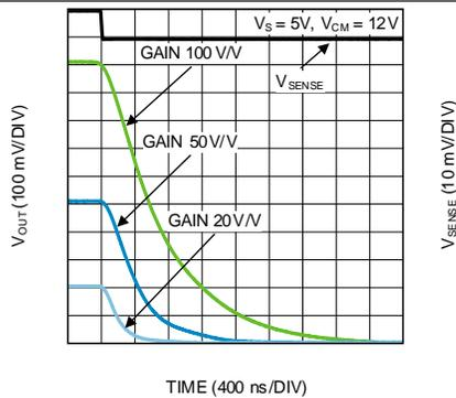
Figure 17. Settling Time (Fall)
