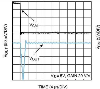
Figure 20. Common Mode Step Response (Fall)
