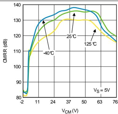
Figure 5. CMRR vs.  $V_{\text{CM}}$  (Gain 20 V/V)
