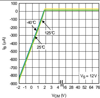
Figure 11.  $I_{\text{Bias}}$  vs.  $V_{\text{CM}}$
