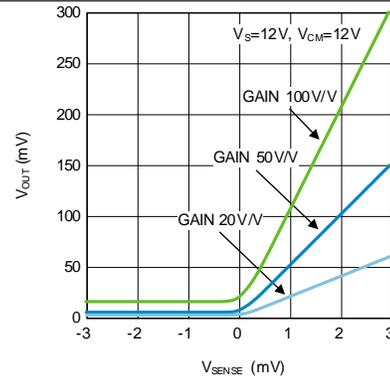
Figure 14. Output Voltage vs.  $V_{\text{SENSE}}$  (ZOOM Close to 0 V)
