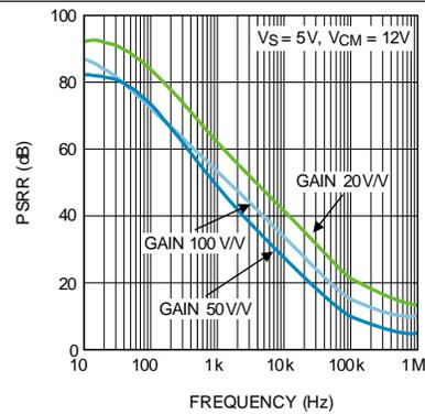
Figure 23. AC PSRR vs. Frequency
