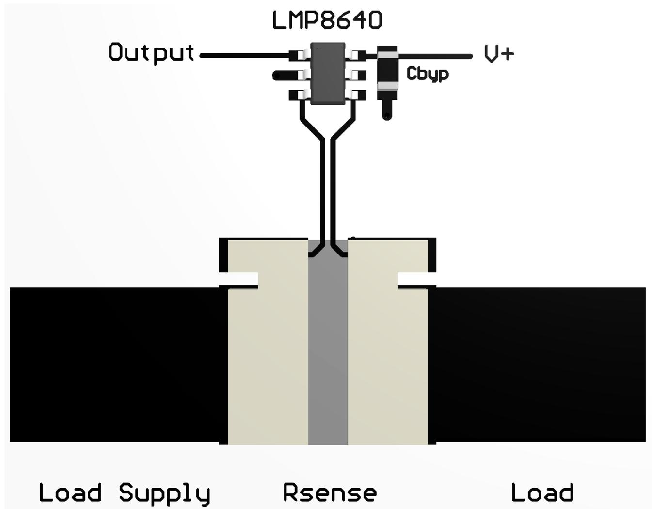
Figure 30. Layout Example - Four-Wire (Kelvin) Resistor Connection
