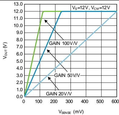
Figure 13. Output voltage vs.  $V_{\text{SENSE}}$
