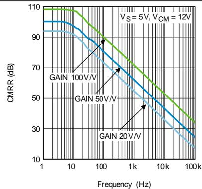
Figure 24. AC CMRR vs. Frequency
