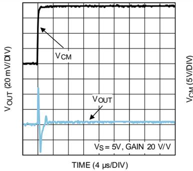
Figure 19. Common Mode Step Response (Rise)
