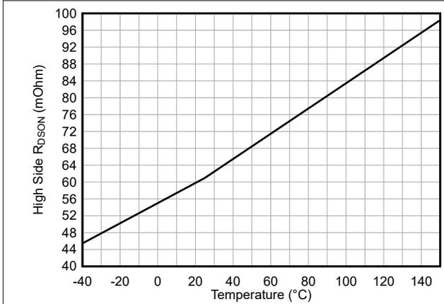
Figure 6-3. High side MOSFET R\_DS-ON
