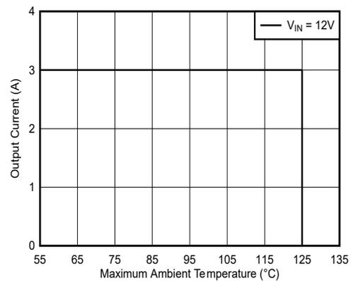
$V_{OUT} = 5V$   $F_{SW} = 400kHz$   $I_{OUT} = 3A$
