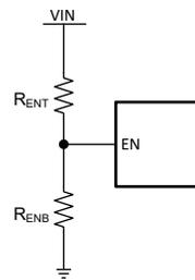
**Figure 7-1. VIN UVLO Using the EN Pin**
