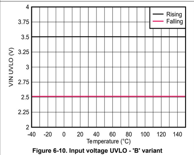
Figure 6-10. Input voltage UVLO - 'B' variant
