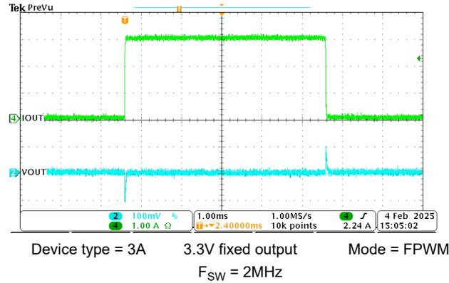
Figure 8-15. 20mA to 3A Load Transient
