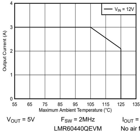
Figure 8-14. Output Current vs Maximum Ambient Temperature
