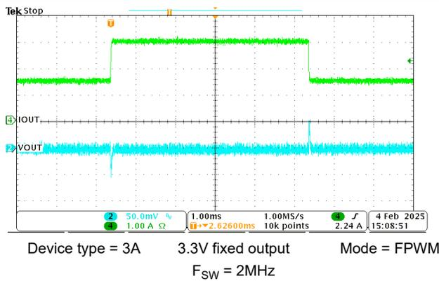
Figure 8-16. 1.5A to 3A Load Transient
