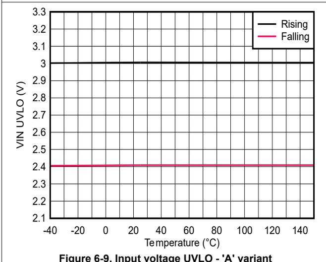
Figure 6-9. Input voltage UVLO - 'A' variant
