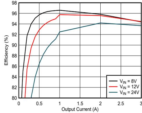
$V_{OUT} = 5V$   $F_{SW} = 400kHz$  Mode = FPWM
