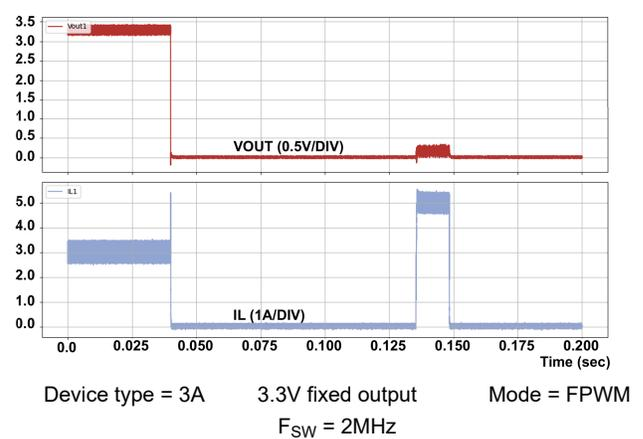
Figure 8-19. Short-Circuit Applied
