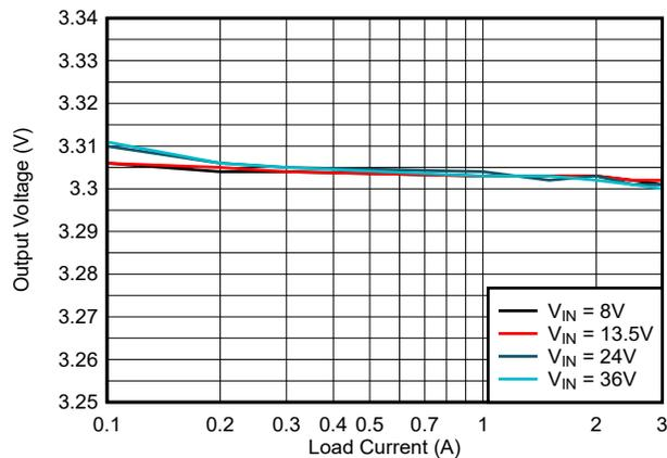
Device type = 3A 3.3V fixed output Mode = Auto
