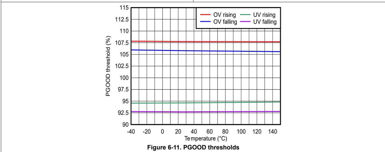
Figure 6-11. PGOOD thresholds
