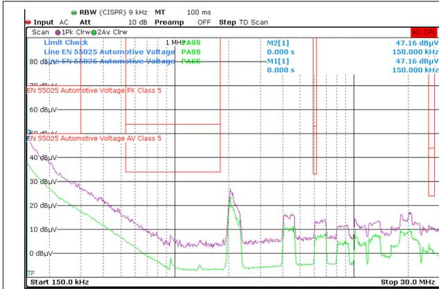
$V_{OUT} = 3.3V$        $F_{SW} = 2MHz$        $I_{OUT} = 3A$
