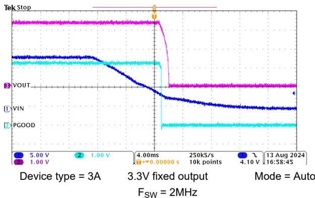
Figure 8-18. Shutdown Operation
