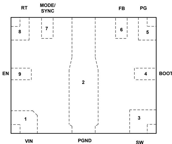
**Figure 5-1. RAK Package 9-Pin WQFN-HR (Top View)**
