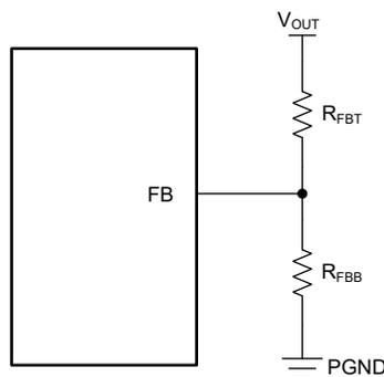
**Figure 7-4. Feedback Resistor Setup for Adjustable VOUT**
