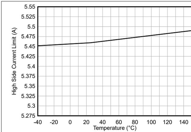
Figure 6-1. High side MOSFET Current Limit
