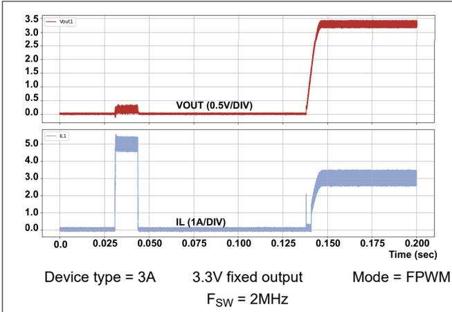
**Figure 8-20. Short-Circuit Recovery**
