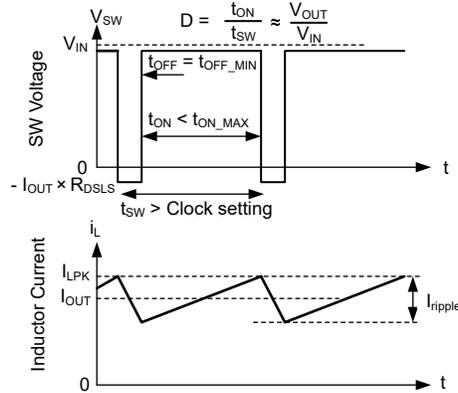
**Figure 7-11. Dropout Waveforms**
