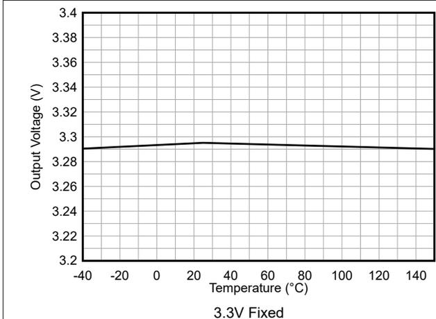
Figure 6-5. Output Voltage Accuracy
