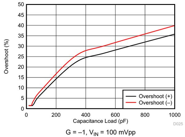
**Figure 6-20. Small Signal Overshoot vs Capacitive Load**
