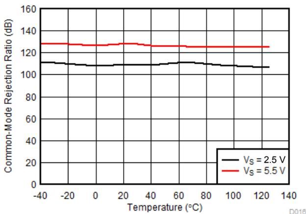
**Figure 6-11. DC CMRR vs Temperature**
