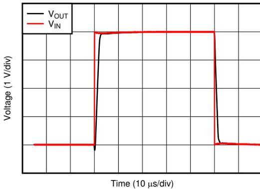
$G = 1$ ,  $V_{IN} = 4\text{ V}_{PP}$ ,  $C_L = 10\text{ pF}$
