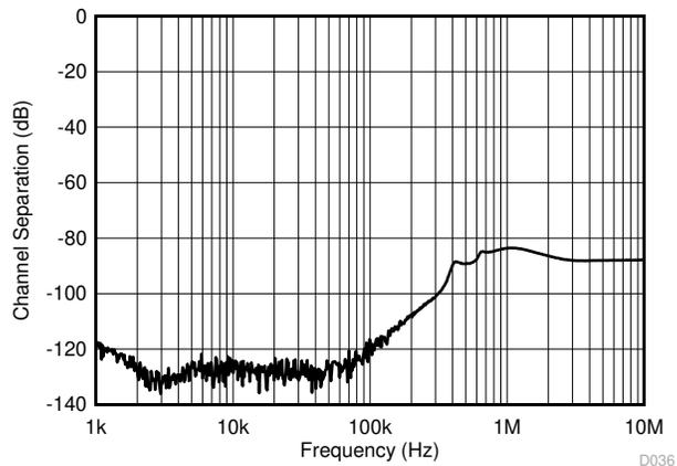
**Figure 6-31. Channel Separation**
