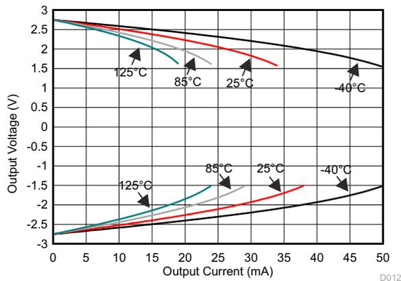
**Figure 6-7. Output Voltage vs Output Current (Claw)**
