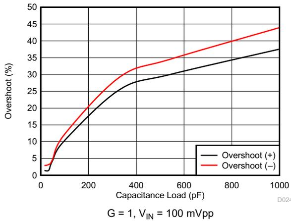
**Figure 6-19. Small Signal Overshoot vs Capacitive Load**
