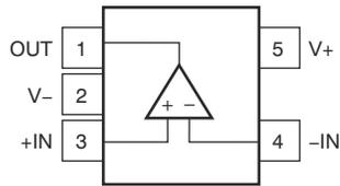
**Figure 5-1. LMV321A-Q1 DBV Package,
