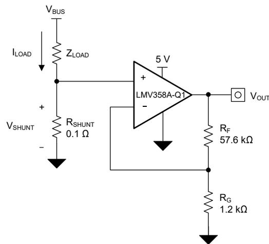
Figure 8-1. LMV3xxA-Q1 in a Low-Side, Current-Sensing Application
