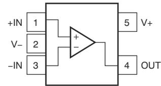
**Figure 5-2. LMV321A-Q1 DCK, LMV321AU-Q1 DBV
