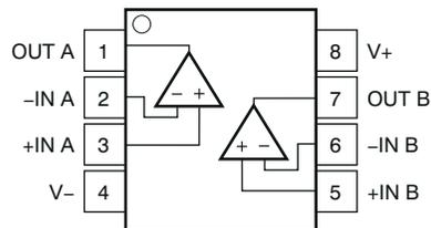
**Figure 5-3. LMV358A-Q1 D and DGK Packages,
