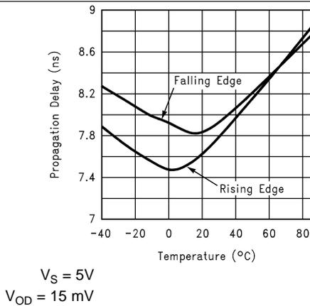
Figure 9. Propagation Delay vs. Temperature
