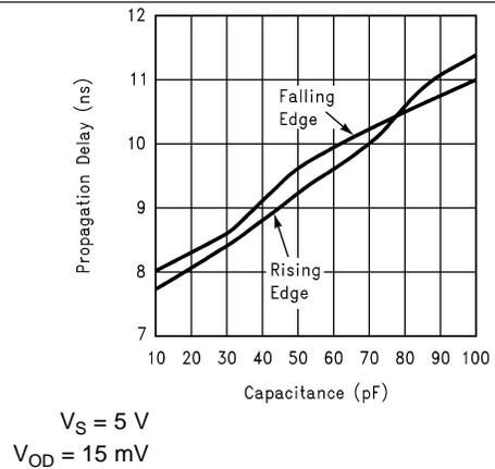
Figure 10. Propagation Delay vs. Capacitive Load
