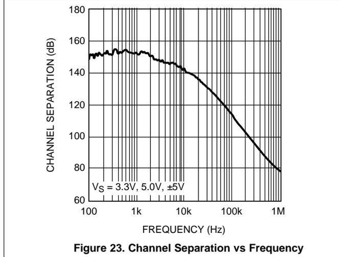
Figure 23. Channel Separation vs Frequency
