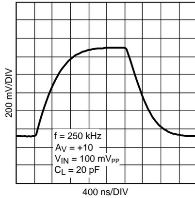
Figure 25. Large Signal Step Response With Gain = 10
