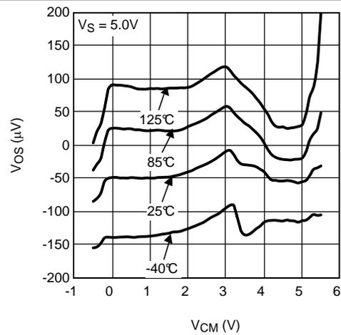
Figure 2.  $V_{OS}$  vs  $V_{CM}$  Over Temperature at 5 V
