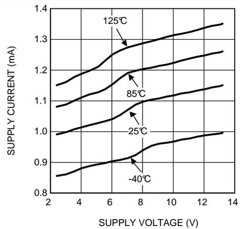
Figure 10. Supply Current Per Channel vs Supply Voltage
