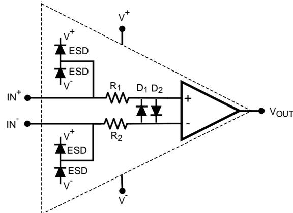
Figure 34. Protection Diodes Between the Input Pins
