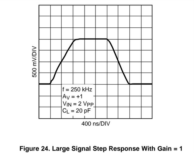
Figure 24. Large Signal Step Response With Gain = 1
