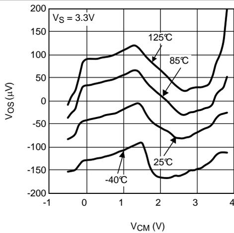
Figure 1.  $V_{OS}$  vs  $V_{CM}$  Over Temperature at 3.3 V
