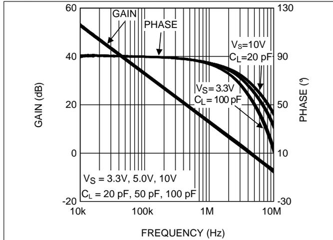
Figure 19. Open-Loop Frequency Response Over Load Conditions
