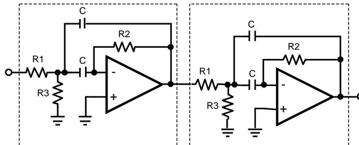
**Figure 38. Active Band-Pass Filter Implementation**
