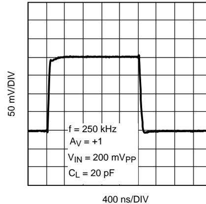
Figure 26. Small Signal Step Response With Gain = 1
