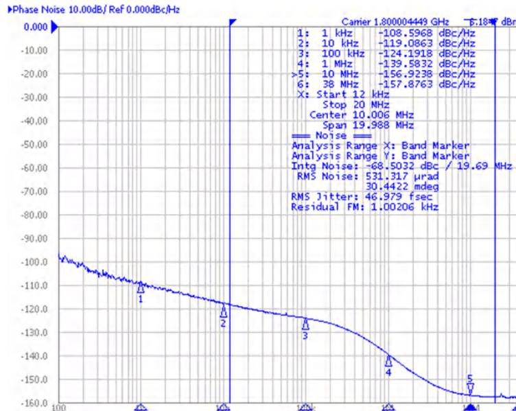
**Figure 8-12. Typical Jitter**
