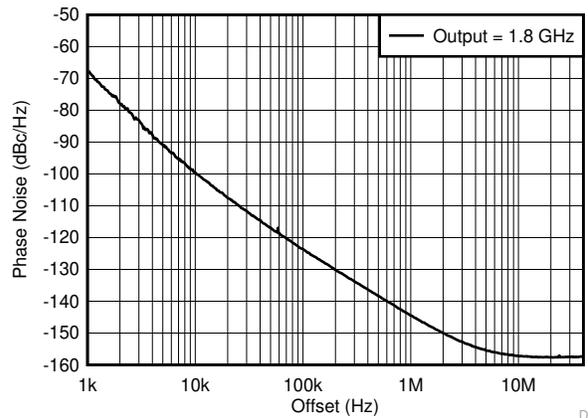
Figure 6-5. 1.8-GHz Output - Open-Loop Phase Noise
