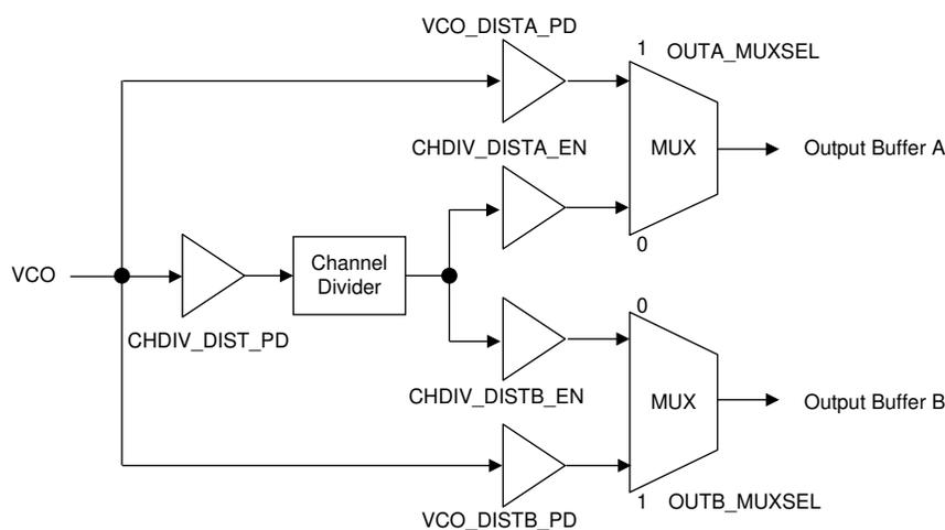
**Figure 7-3. Output Distribution Diagram**
