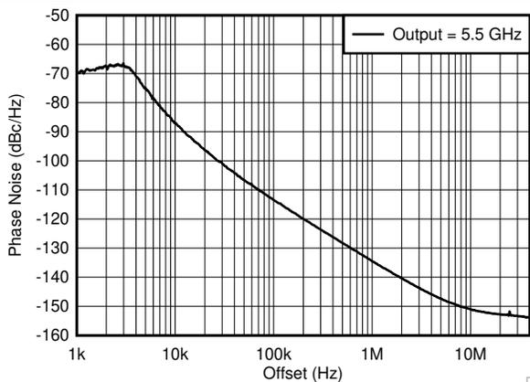
Figure 6-6. 5.5-GHz Output - Closed-Loop Phase Noise
