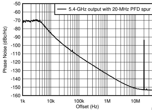
Figure 6-14. Typical PFD Spur for 5.4-GHz Output
