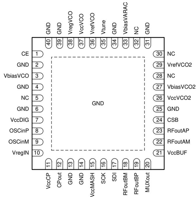
Figure 5-1. RHA Package 40-Pin VQFN Top View
