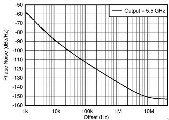
Figure 6-7. 5.5-GHz Output - Open-Loop Phase Noise
