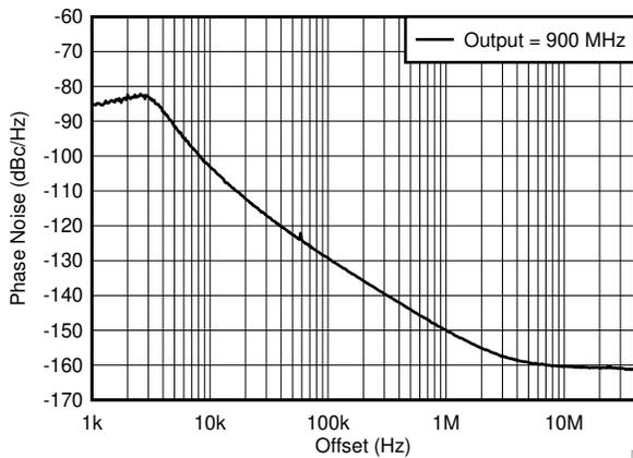
Figure 6-2. 900-MHz Output - Closed-Loop Phase Noise
