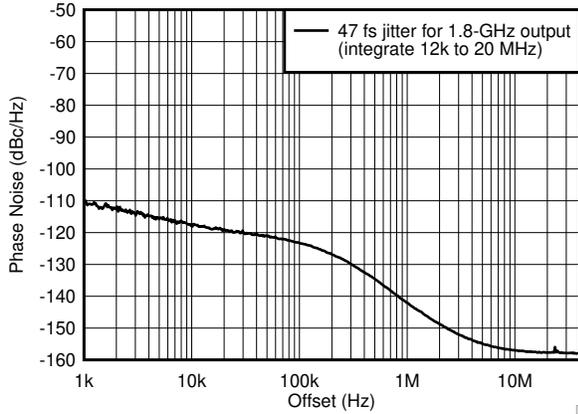
**Figure 6-8. Integrated Jitter (47 fs) - 1.8-GHz Output**
