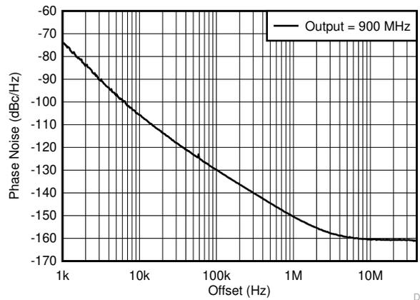
Figure 6-3. 900-MHz Output - Open-Loop Phase Noise
