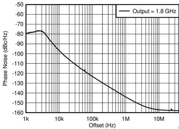
Figure 6-4. 1.8-GHz Output - Closed-Loop Phase Noise
