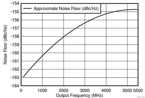
Figure 6-17. Noise Floor Variation With Output Frequency
