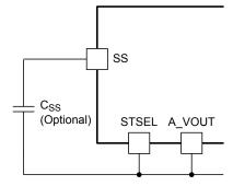
Figure 45. Slow-Start Capacitor (C<sub>SS</sub>) and STSEL Connection
