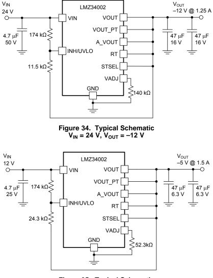
Figure 35. Typical Schematic  $V_{IN}$  = 12 V,  $V_{OUT}$  = -5 V
