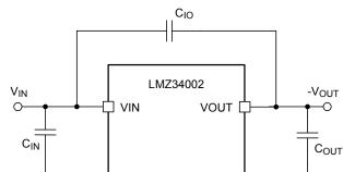
Adding an input to output coupling capacitor ( $C_{IO}$ ) across VIN to VOUT as shown in Figure 46 can help reduce output voltage ripple and improve transient response. A typical value for  $C_{IO}$  is 2.2 µF ceramic with a voltage
