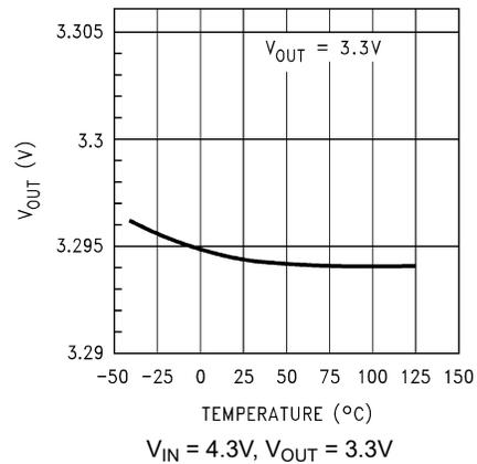
Figure 5-2. Output Voltage vs Temperature (Legacy Chip)
