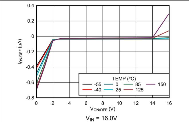
Figure 5-56.  $\text{ON}/\overline{\text{OFF}}$  Pin Current vs  $V_{\text{ON}/\overline{\text{OFF}}}$  (New Chip)
