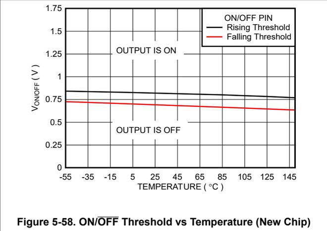
Figure 5-58.  $\text{ON}/\overline{\text{OFF}}$  Threshold vs Temperature (New Chip)
