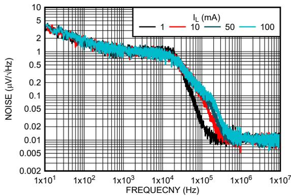
**Figure 5-45. Output Noise Density vs Load Current ( $I_L$ ) Frequency (New Chip)**
