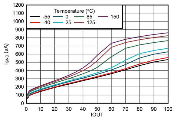
Figure 5-18. Ground Pin Current ( $I_{GND}$ ) vs Load Current (New Chip)
