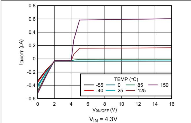
Figure 5-55.  $\text{ON}/\overline{\text{OFF}}$  Pin Current vs  $V_{\text{ON}/\overline{\text{OFF}}}$  (New Chip)
