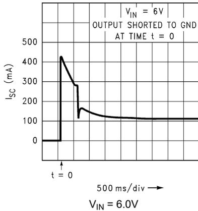
Figure 5-31. Short-Circuit Current vs Time (Legacy Chip)
