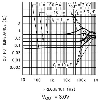
**Figure 5-39. Output Impedance vs Frequency (Legacy Chip)**
