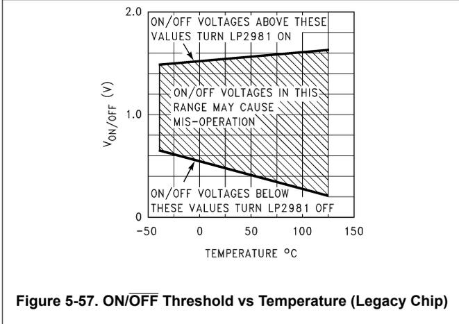
Figure 5-57.  $\text{ON}/\overline{\text{OFF}}$  Threshold vs Temperature (Legacy Chip)
