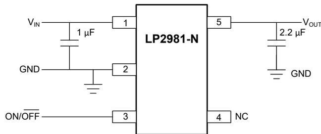
\*The ON/OFF input must be actively terminated. Tie to  $V_{IN}$  if this function is not to be used. Minimum output capacitance is shown to provide stability over full load current range. More capacitance provides superior dynamic performance and additional stability margin (see the [Recommended Capacitor Types](#) section).
