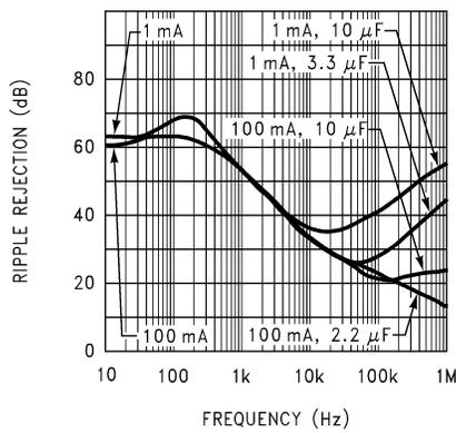
**Figure 5-41. Ripple Rejection vs Frequency (Legacy Chip)**
