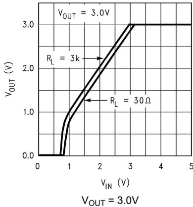
Figure 5-7. Output Voltage vs  $V_{IN}$  (Legacy Chip)
