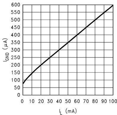
Figure 5-17. Ground Pin Current ( $I_{GND}$ ) vs Load Current (Legacy Chip)
