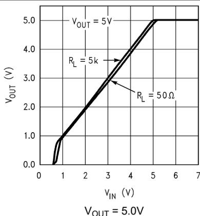
Figure 5-5. Output Voltage vs  $V_{IN}$  (Legacy Chip)
