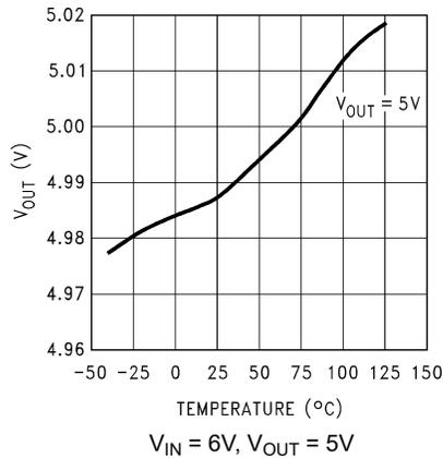
Figure 5-1. Output Voltage vs Temperature (Legacy Chip)
